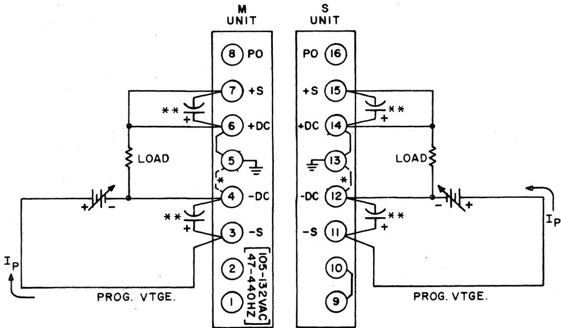
NOTE: VOLTAGE ADJ. CONTROLS MUST BE SET TO MINIMUM OUTPUT VOLTAGE.
