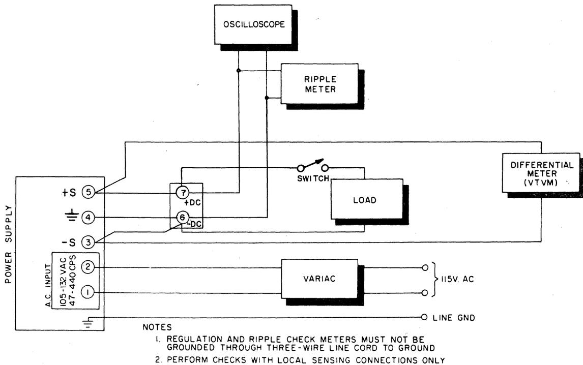
Figure 9. Test Connections for Performance Checks
