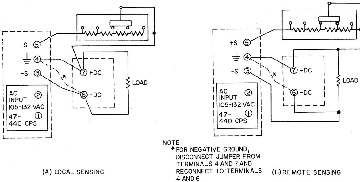
Figure 5. Programmed Voltage, with External Resistor
