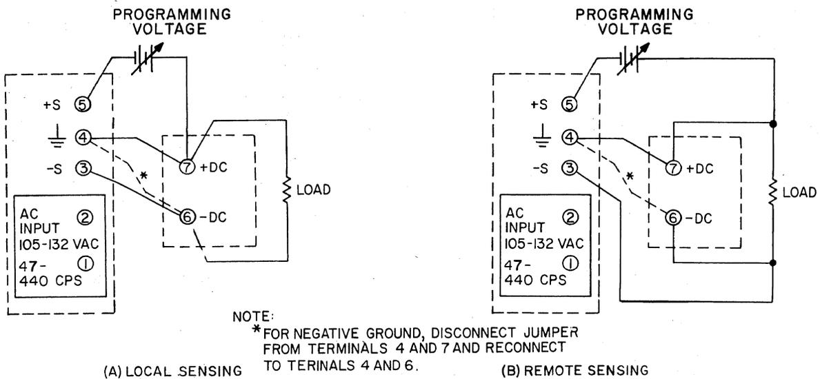
Figure 6. Programmed Voltage, with External Programming Voltage Source
