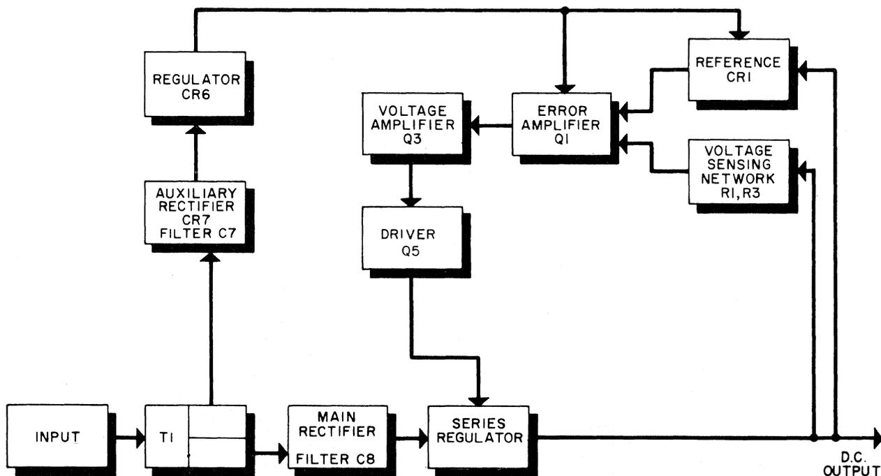
Figure 7. Typical Block Diagram
