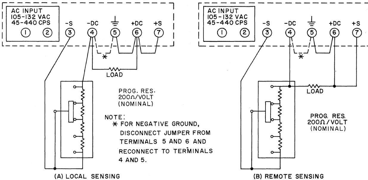
Figure 5. Programmed Voltage, with External Resistor
