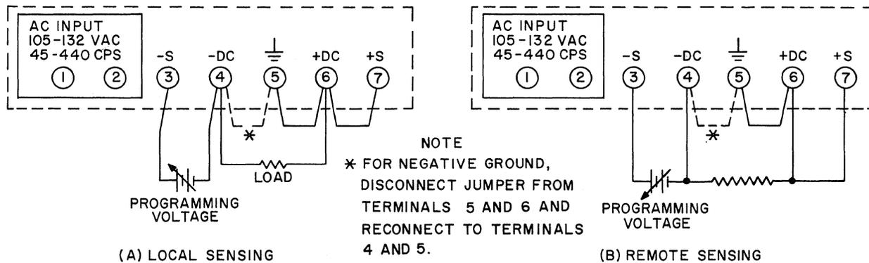
Figure 6. Programmed Voltage, with External Programming Voltage Source
