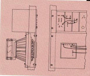
The BD-100 Series may be panel or deck mounted in any orientation and is available as a bench unit. Connections to the heads or associated electronics may be made through connectors in permanent installations, or through a convenient patch-cord plug-board for system mock-ups.
