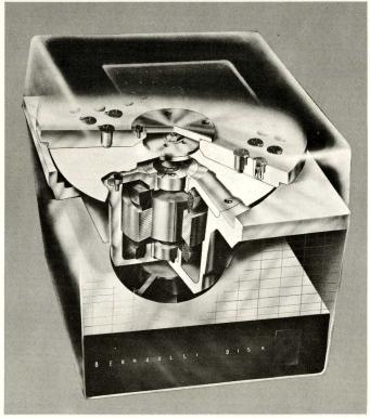
The BERNOULLI DISK . . . . simplest rotating storage device ever developed . . . small and compact . . . wide application in fixed station and mobile digital computers.
