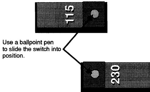
**Figure 1-3. Line Voltage Switch Settings**
