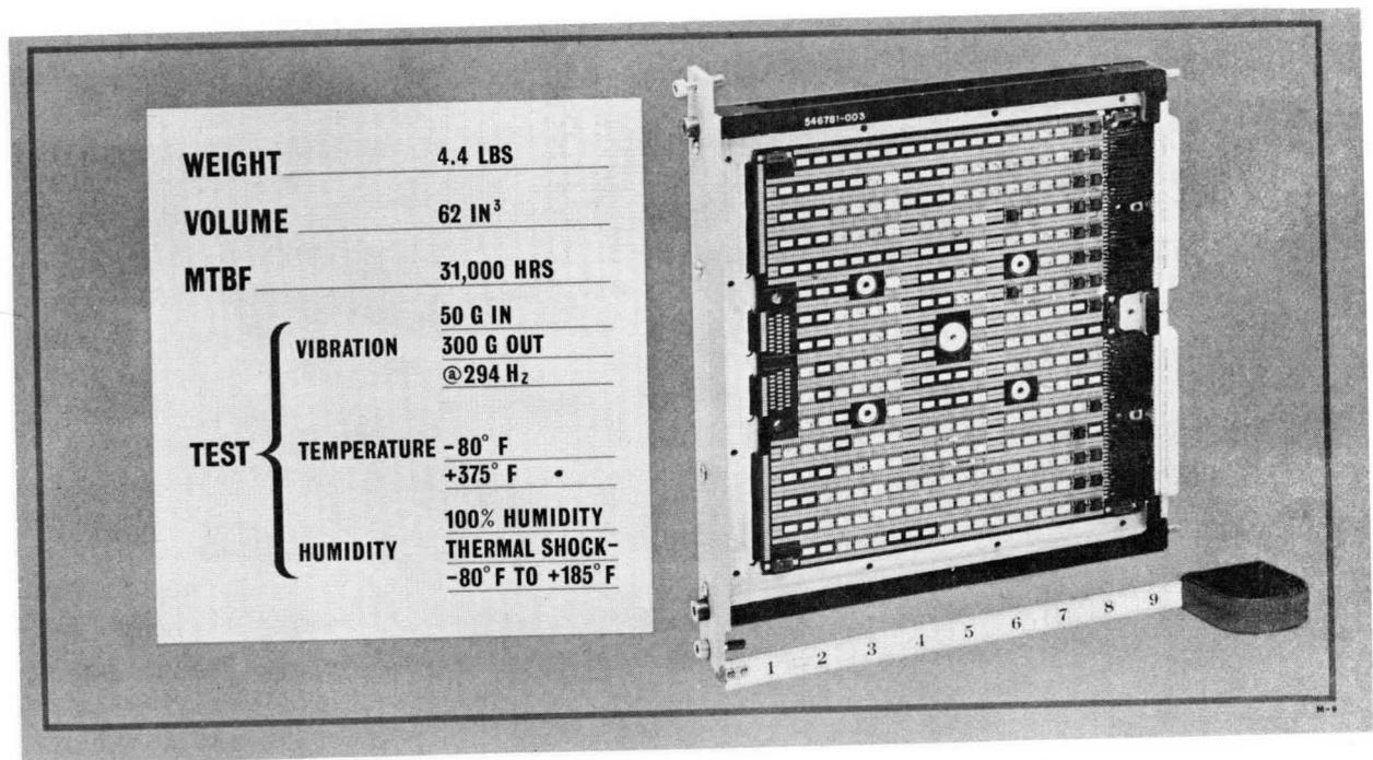
Figure 22. Arithmetic and Control Module Parameters
