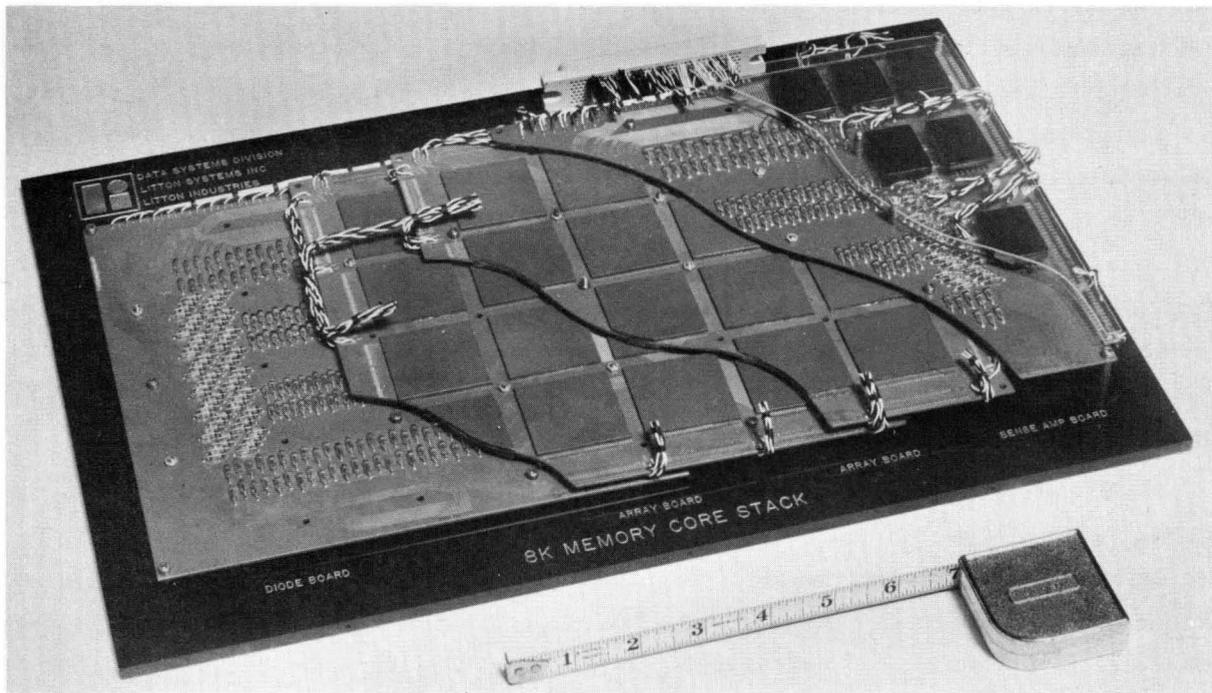
Figure 18. Exploded 8192-Word Memory Core Stack
