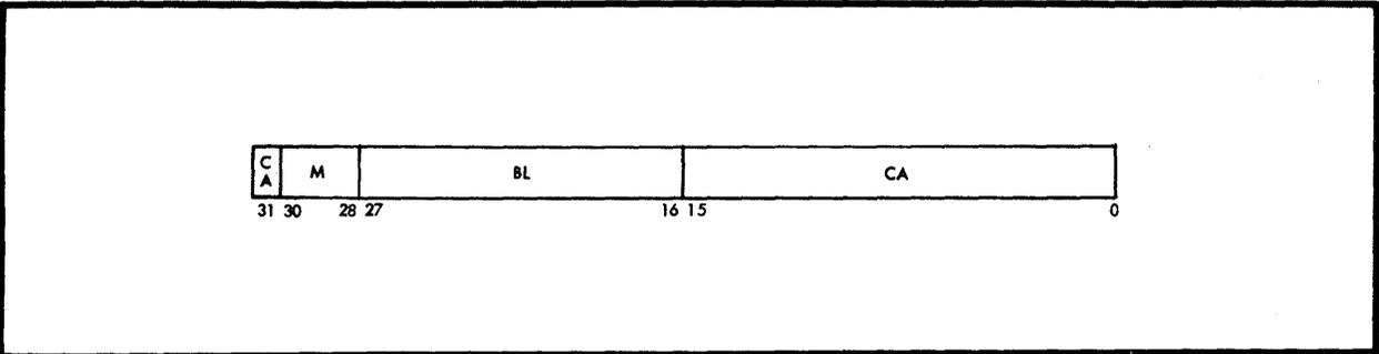
Figure 4. Input/Output Key Word Format
