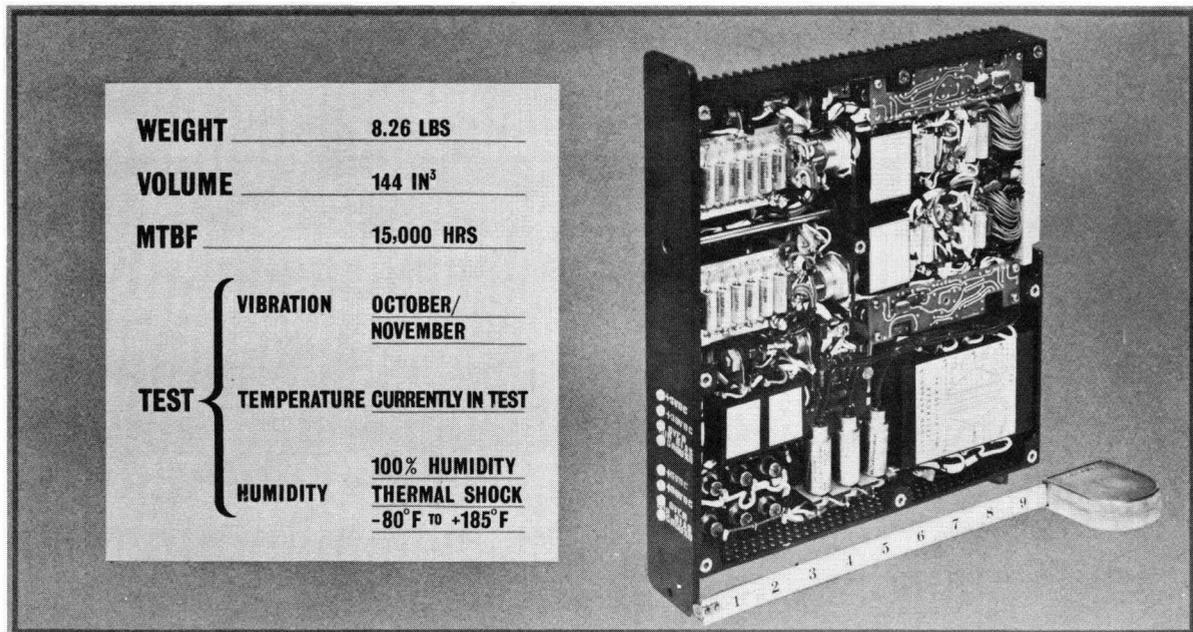
Figure 25. Power Supply Drawer Parameters
