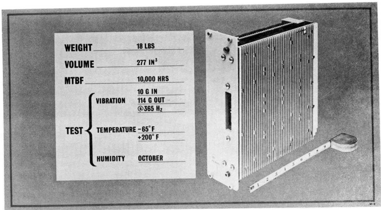
Figure 21. Memory Module Verified Parameters
