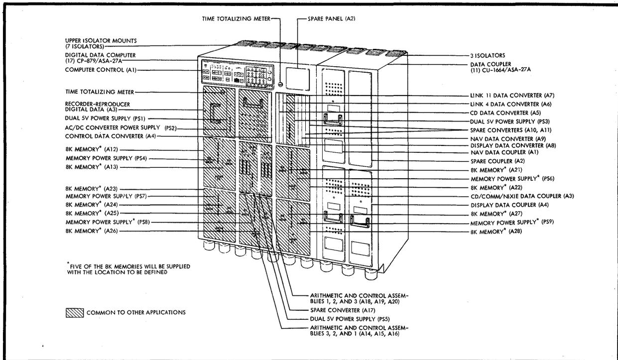
Figure 13. Data Processor Layout
