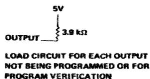
FIGURE 1 – LOAD CIRCUIT
