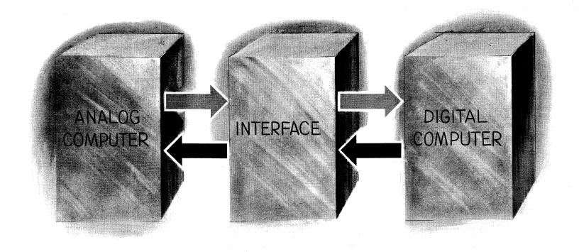
First, I think I should tell you what a hybrid computer is. A hybrid computer is composed of an analog computer, an interface system, and a digital computer. What we have to do is to constrain these three diverse pieces of equipment to work as a single system.
