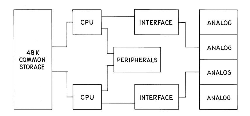
The particular hybrid system that we have conceived to handle the problem posed by the C3 Project consists of two central processing units connected to a common core storage of approximately 48,000 words. They are connected to the normal digital peripheral equipment, two pieces of interface equipment and four analog computers.
