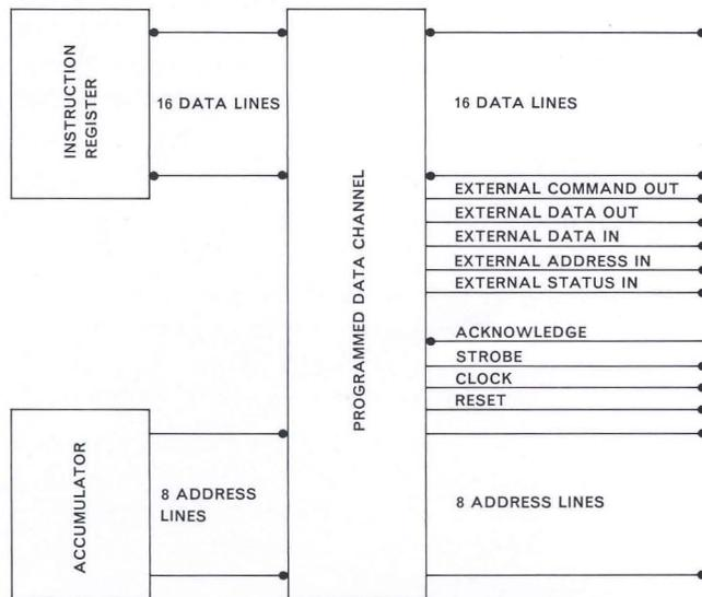
The PDC is controlled by five instructions: Data In, Data Out, Address In, Command Out, and Status In. Each instruction is identified by a single line in the PDC to minimize decoding in peripheral device controllers.
