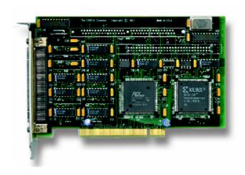
**Provides a migration path**. The BCI-2104 allows users of Q-bus systems to migrate to VAX and PDP-11 emulators and retain their existing Q-bus I/O devices without loss of function or performance.
