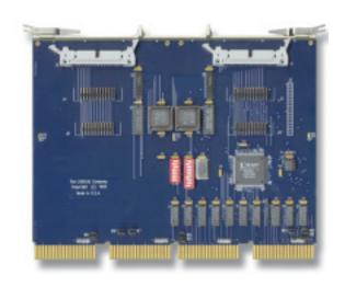
The DCQ-3100 is a DMA controller that interfaces a Q-bus system to two independent channels that are compatible with both the IEC and IEEE instrument buses. The instrument buses conform to both the European Standard IEC 625-1 and the U.S. Standard IEEE 488.1-1987. Each instrument bus can have up to fifteen devices, including the DCQ-3100, in a sequential configuration.
