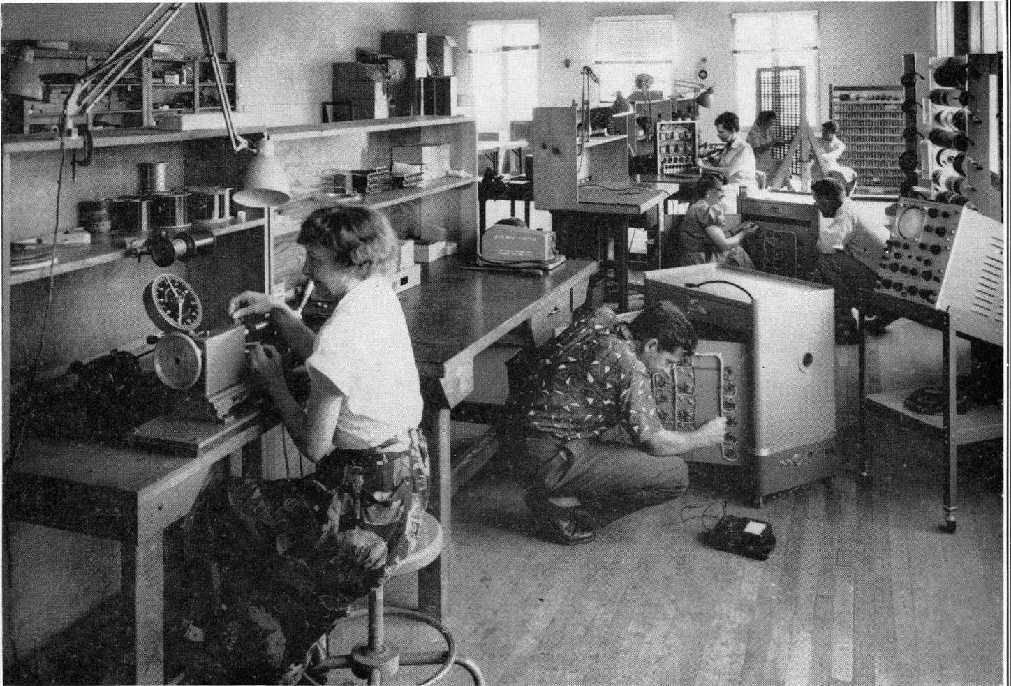
This is the Sub-Assembly Area of the main assembly room where plug-in components are constructed, special coils wound, and various small electronic units are assembled. In the rear at the far right can be seen the frameworks for two ALWAC Logic sections.
