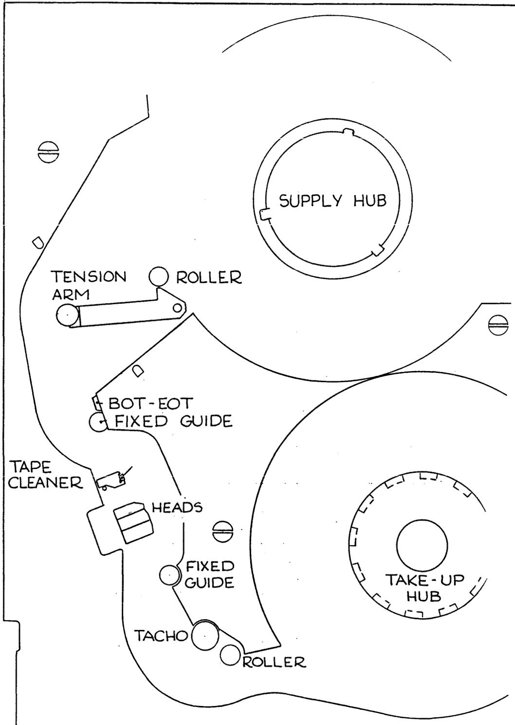
FIGURE 5.1 TAPE PATH COMPONENTS
