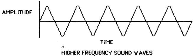
Longer strings produce low tones while shorter strings produce higher tones. So that instruments may play together harmoniously, each is designed so that it can produce tones of a certain frequency of vibration or pitch.
