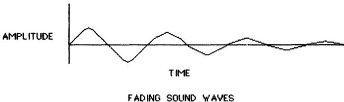
If the string is plucked more forcefully (pulled farther from its rest position) a different intensity or *volume* of sound is heard. Thus, the volume of the tone depends on the amplitude of the vibration.
