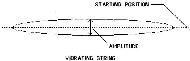
This process continues until friction causes the amplitude of the vibration to diminish until we can no longer hear the sound.
