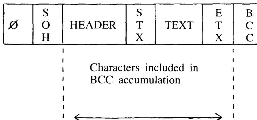
*Figure 3. Block-Check Character Accumulation for Entire Transmission*
