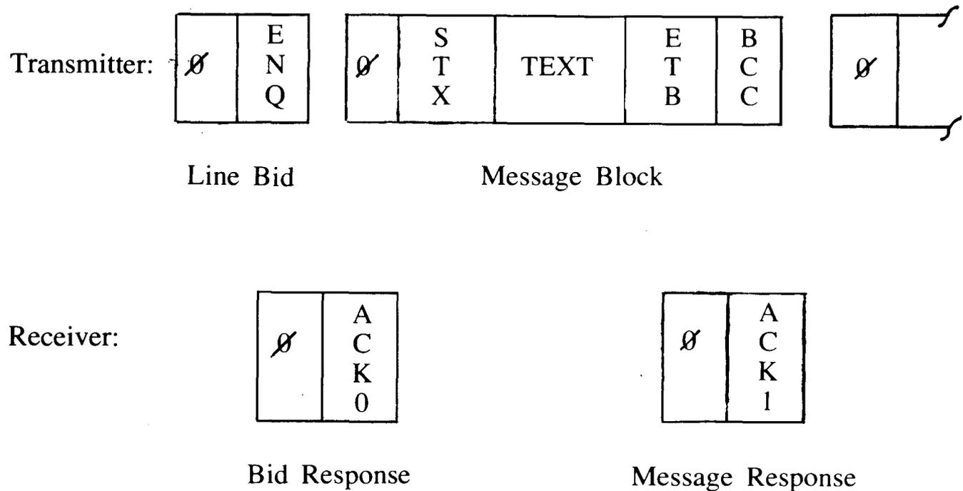
*Figure 4. Line Bid Processing (Point-to-Point Operation)*
