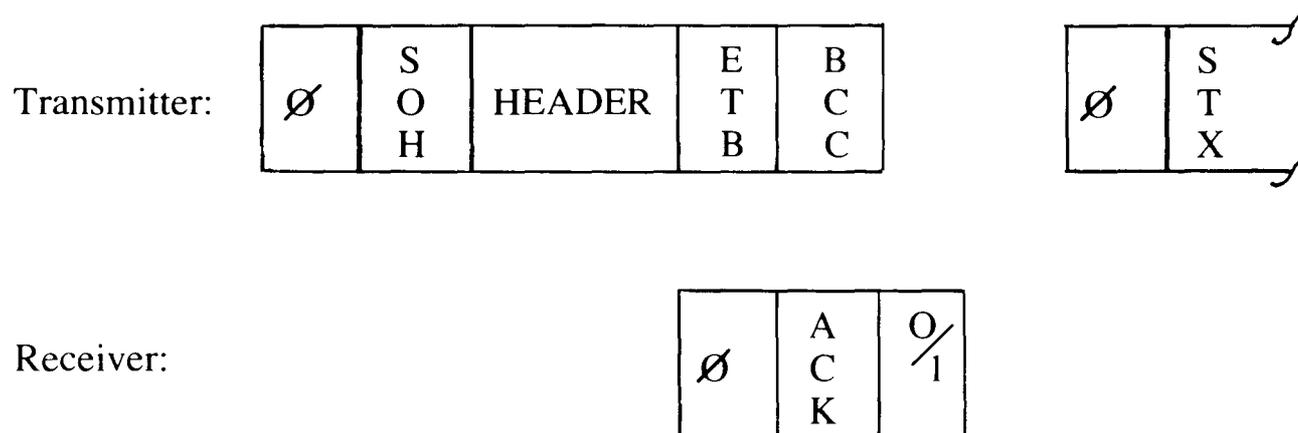
*Figure 2. Header Terminated by ETB for Error Checking Purposes*
