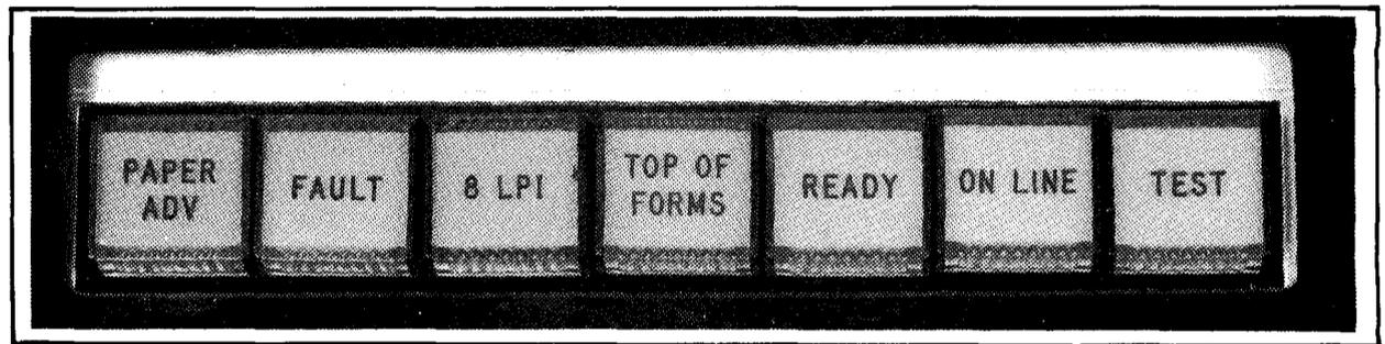
Figure 2-2. Printer Controls.
