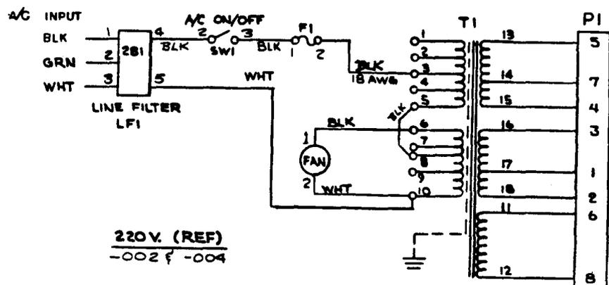
Figure 2-2. Converting From 100V to 220V
