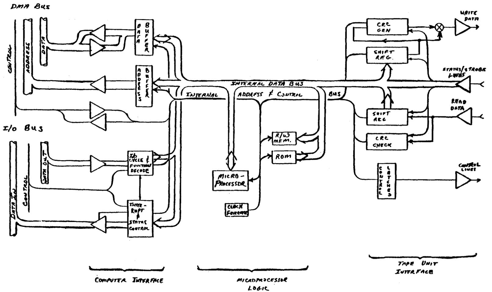
Figure A3-1. Cartridge Tape Controller Block Diagram
