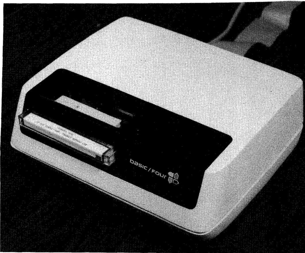
Figure 1-1. Magnetic Tape Cartridge Drive (MTCD)
