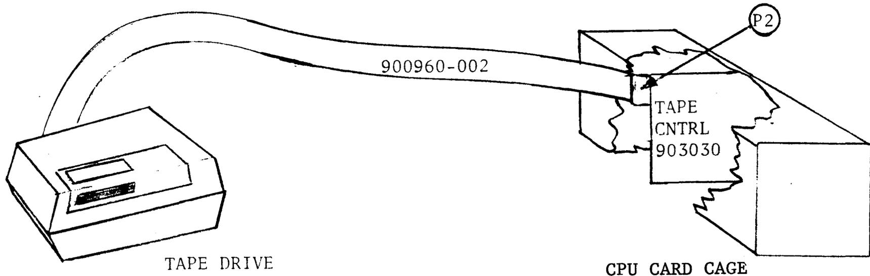
Figure A1-1. Magnetic Tape Cartridge/Controller Interface Cabling
