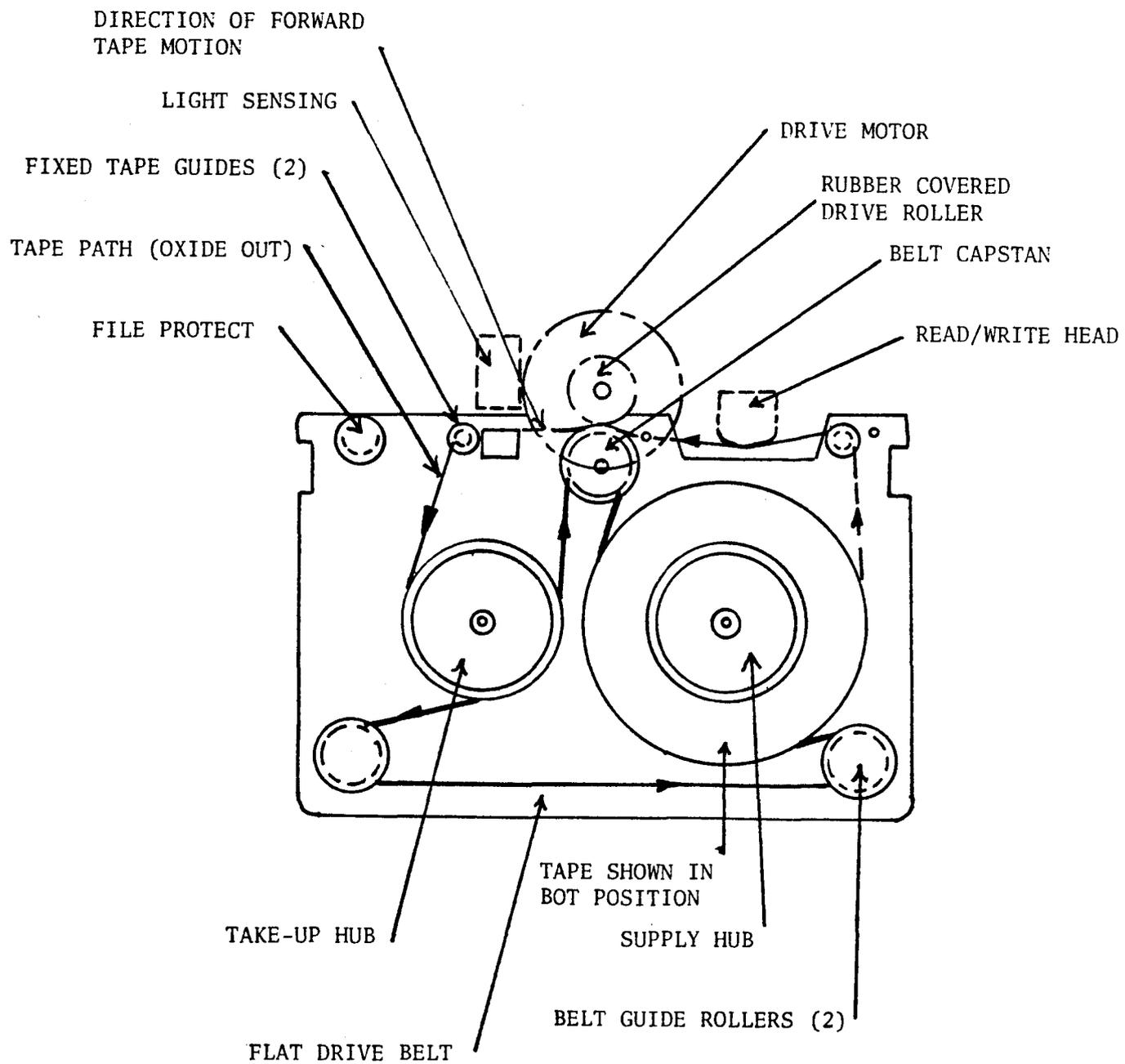
Figure 1-5. Cartridge Diagram
