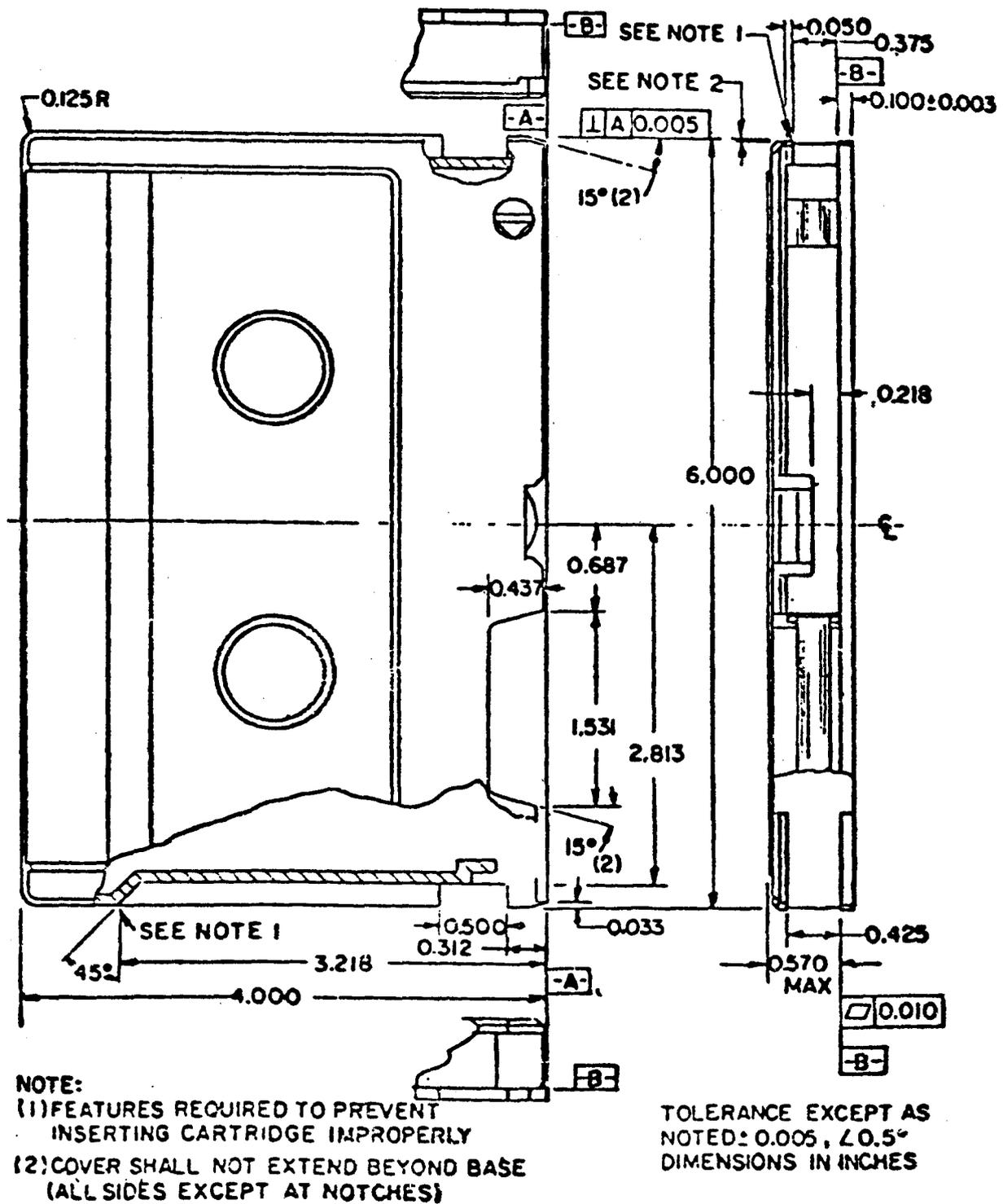
Figure 1-6. Cartridge Dimensions
