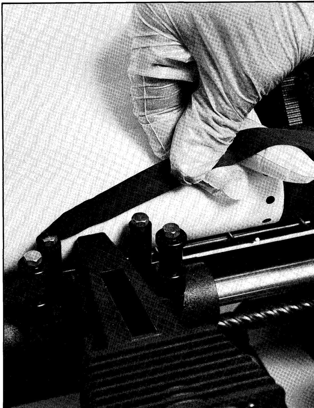
*Figure 56. Threading ribbon around printer head*
