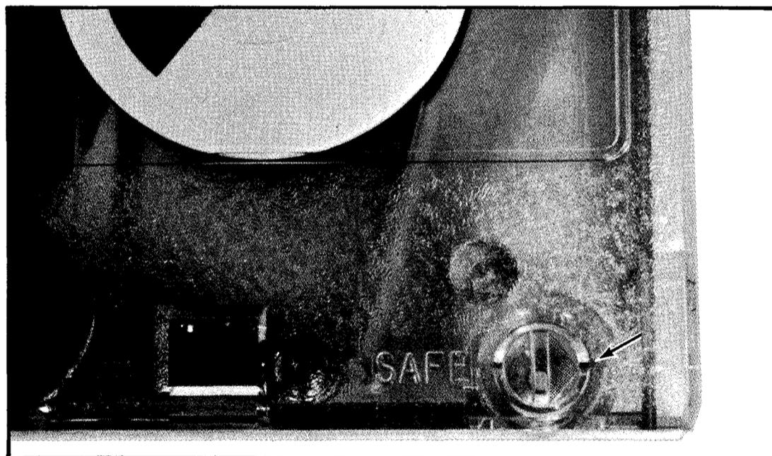
*Figure 12. Tape cartridge safety lock off (read-write position)*
