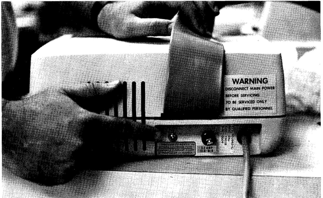
Figure 3-11. Tape cartridge drive power switch
