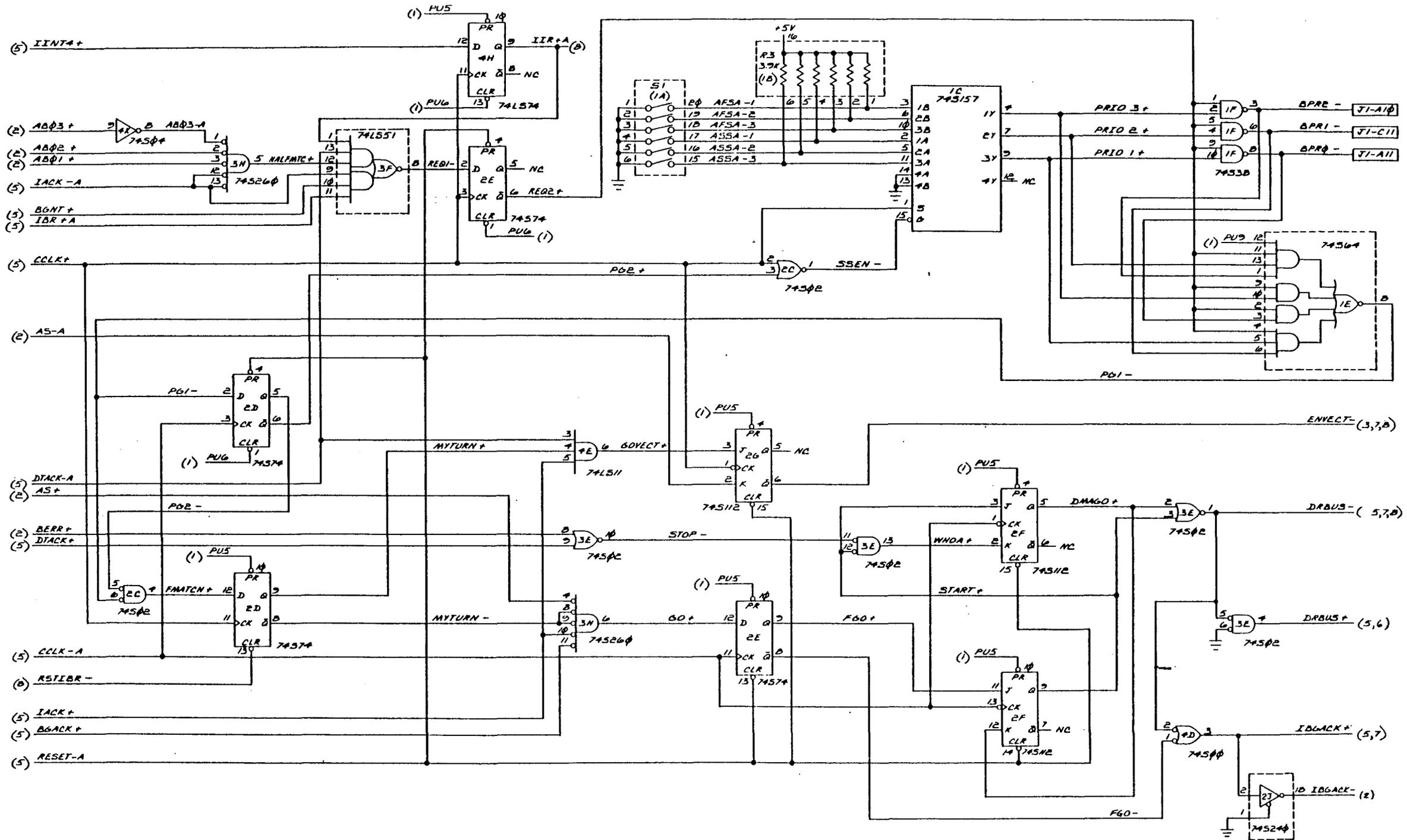
Figure 7-1. 4-Way Controller PCB - Logic Diagrams (Sheet 5 of 10)
