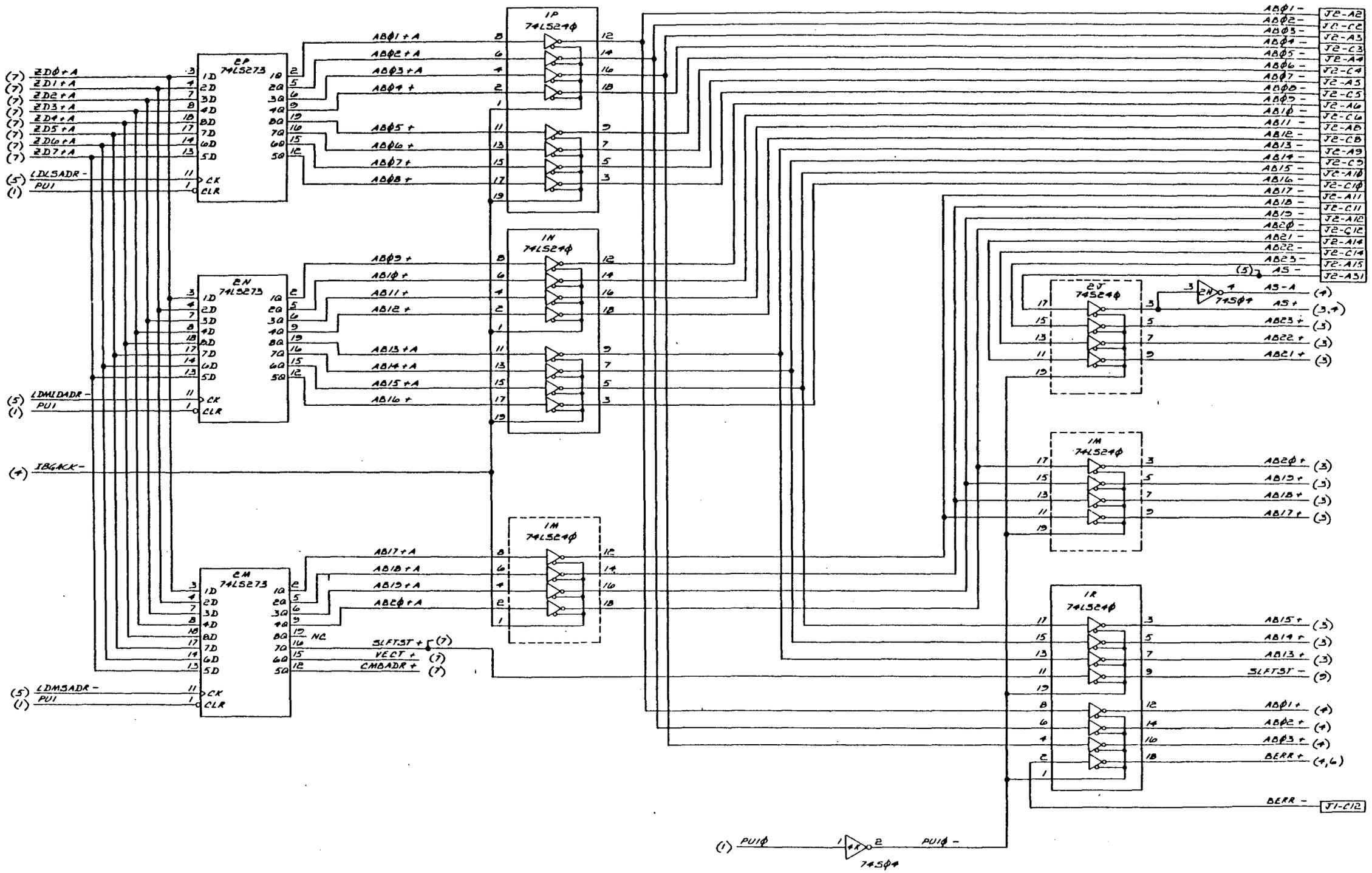
Figure 7-1. 4-Way Controller PCBA - Logic Diagrams (Sheet 3 of 10)
