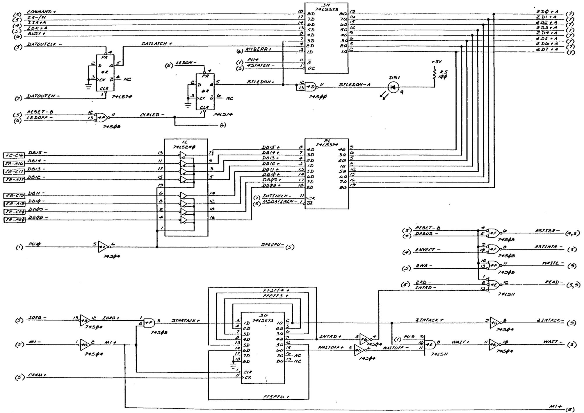
Figure 7-1. 4-Way Controller PCBA - Logic Diagrams (Sheet 10 of 10)
