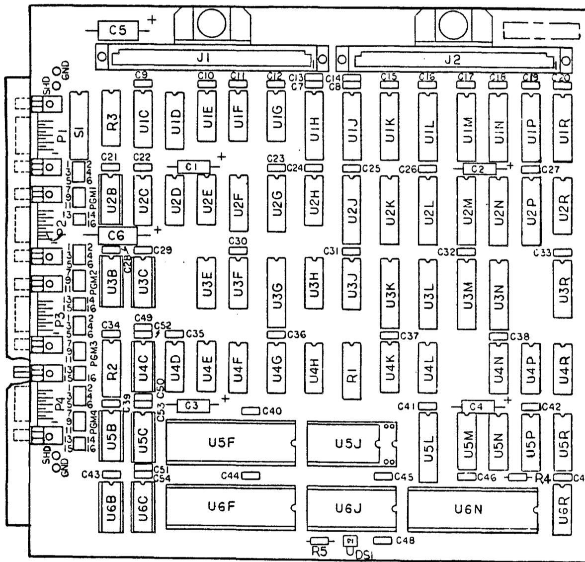
Figure 1-1. 4-Way Controller PCBA - Part No. 903390
