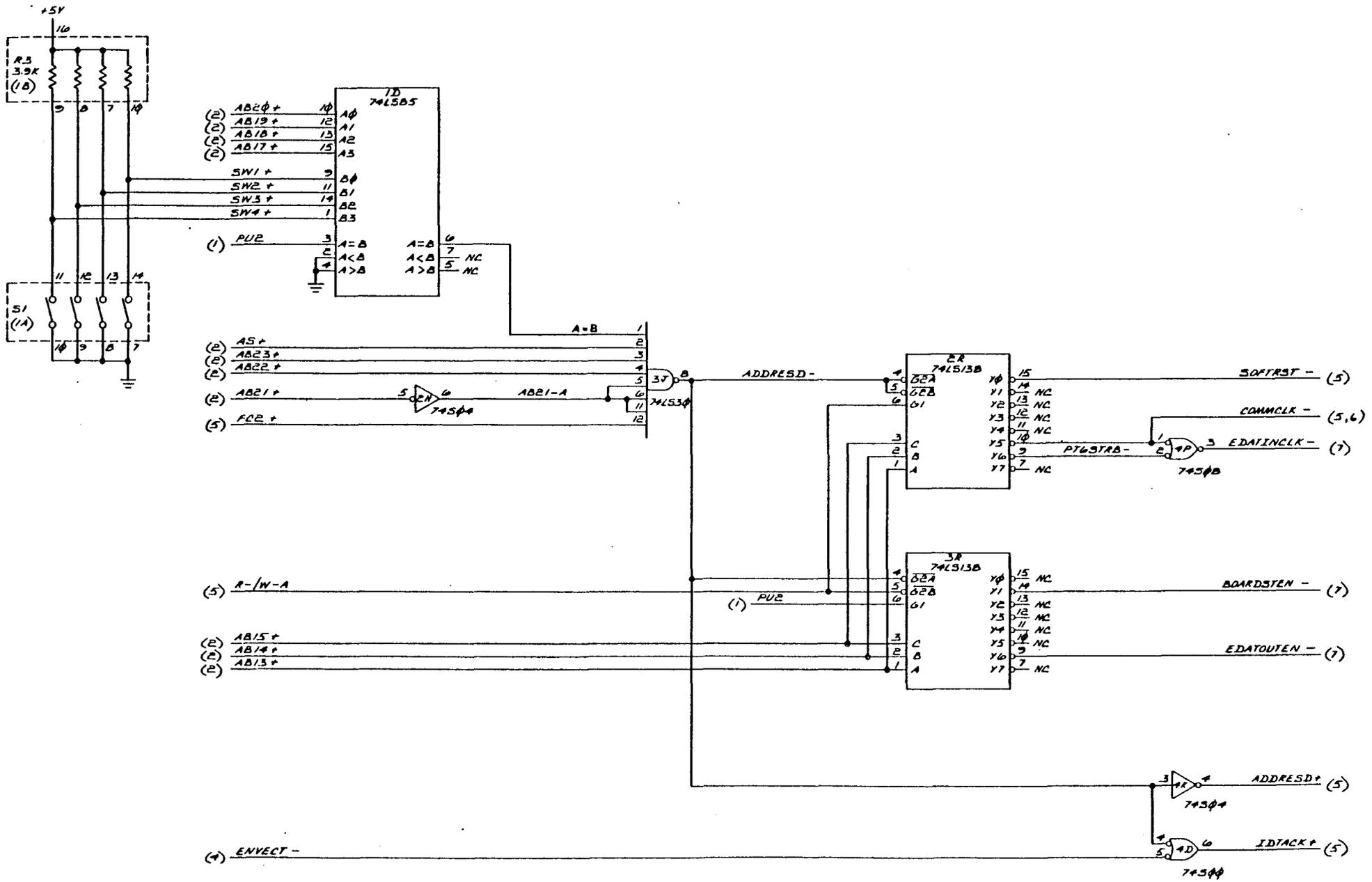
Figure 7-1. 4-Way Controller PCB A - Logic Diagrams (Sheet 4 of 10)
