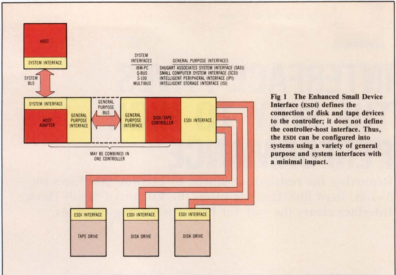
**Fig 1 The Enhanced Small Device Interface (ESDI) defines the connection of disk and tape devices to the controller; it does not define the controller-host interface. Thus, the ESDI can be configured into systems using a variety of general purpose and system interfaces with a minimal impact.**
