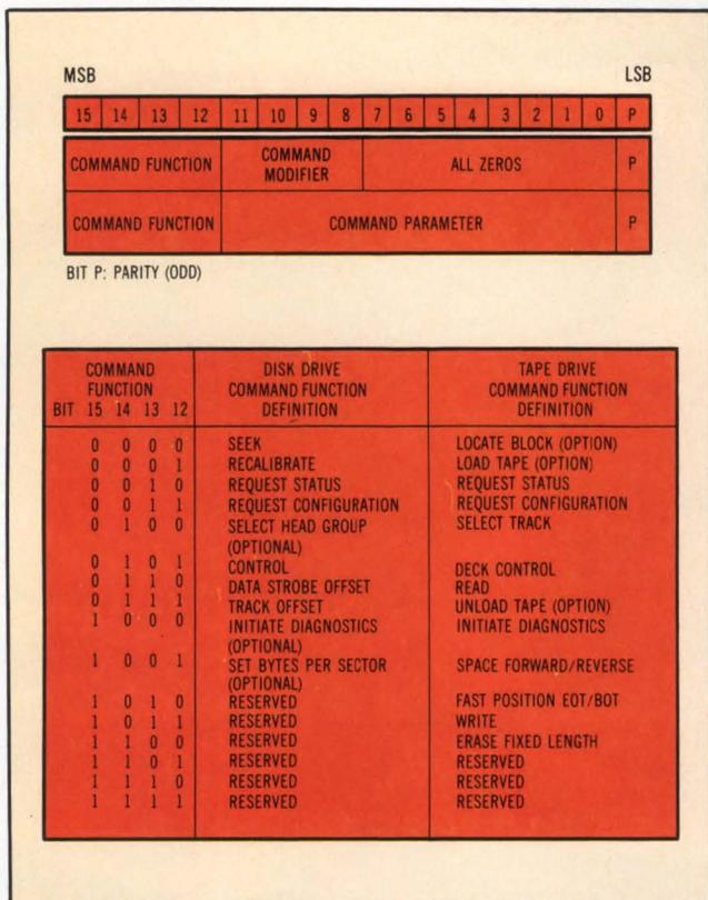
**Fig 3** The serial mode of implementation for disk and tape devices takes advantage of added drive intelligence. Communications with the drive are carried out through 16-bit commands and responses, followed by a parity bit. Thus, the system can be self-configuring, simplifying the writing of software to handle a wide variety of devices.
