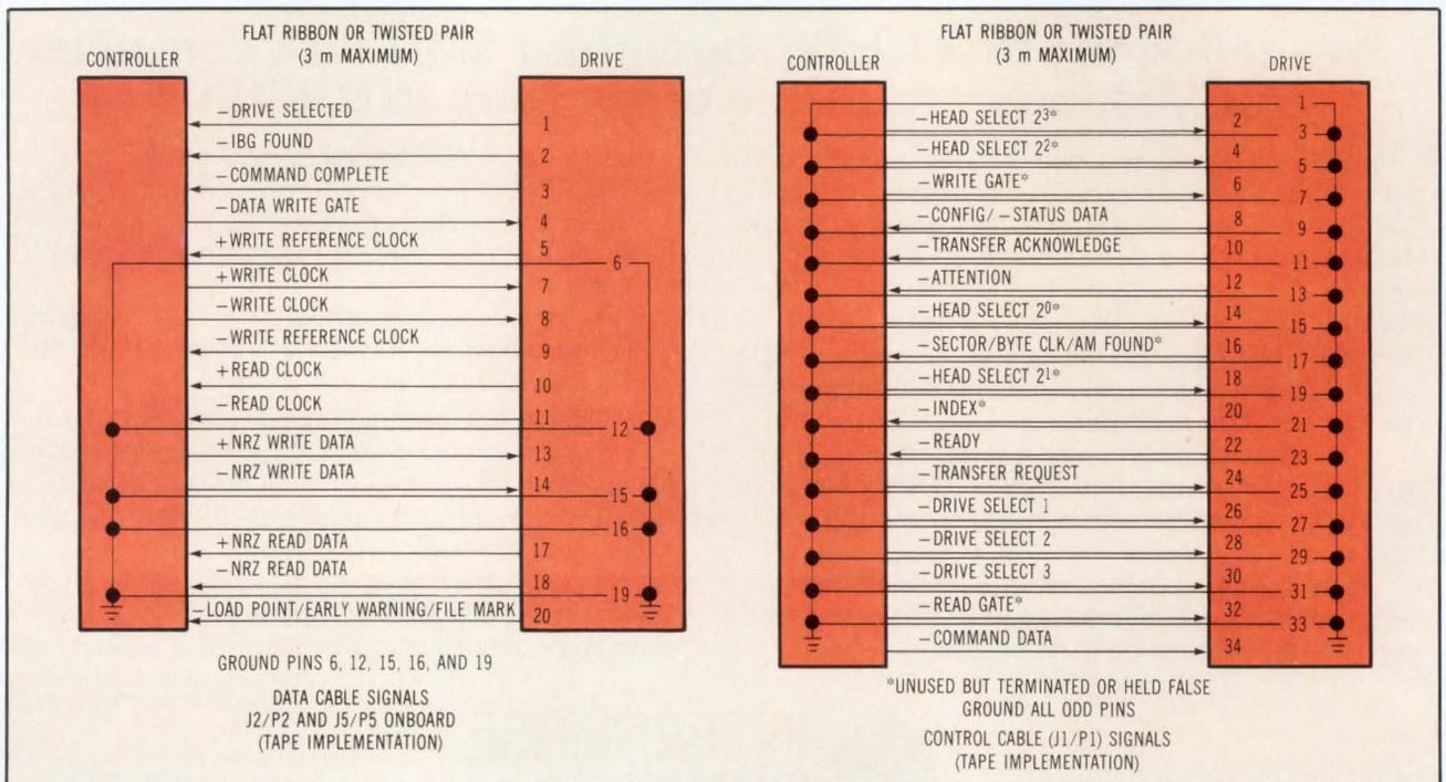
**Fig 5** In ESDI tape implementation, pin assignments differ slightly from those used for disk implementations. Only serial mode is supported, and a write reference clock has been added to allow read after write operation.
