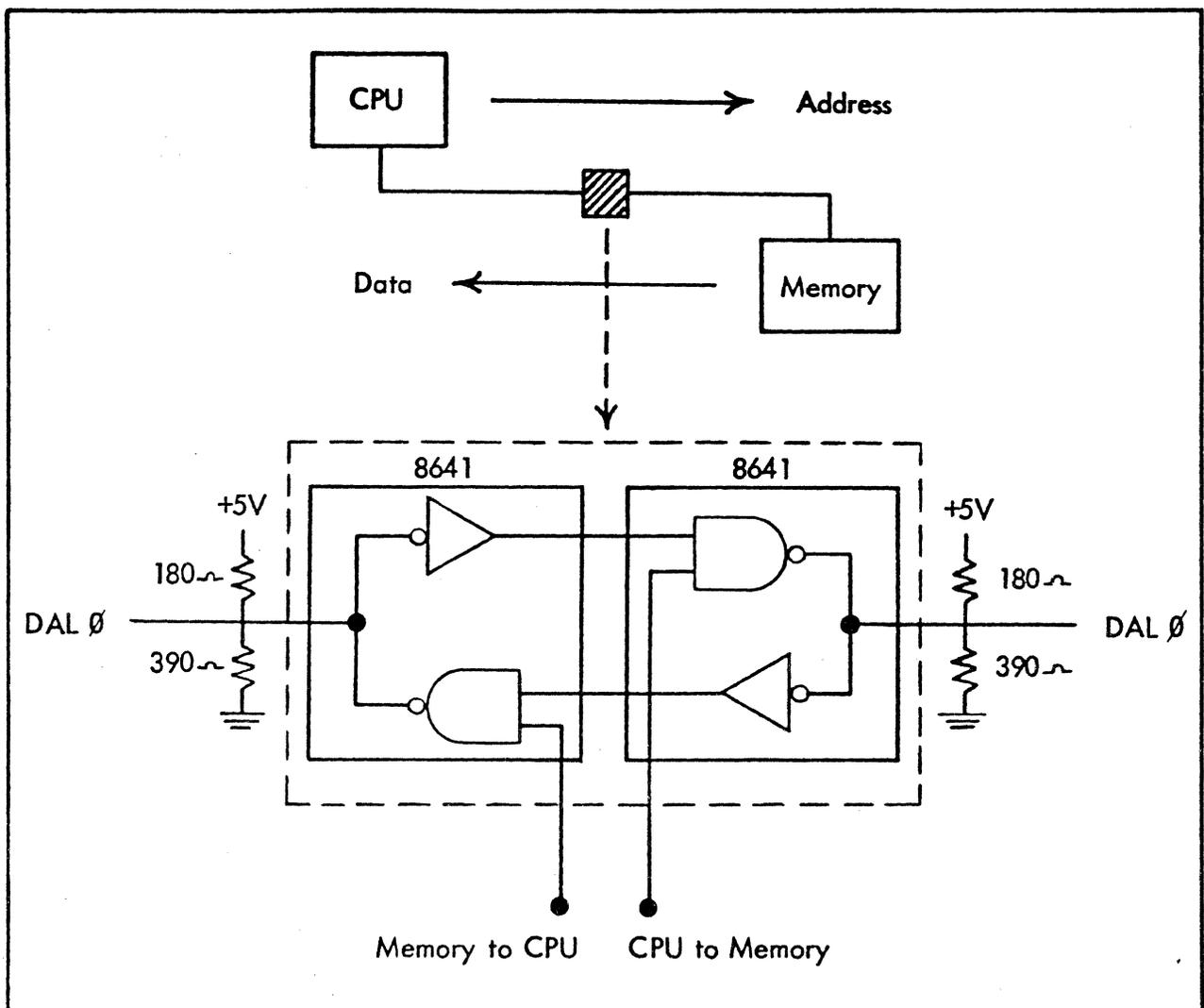
When the Bus Repeater is inserted into the system between the processor and memory (as shown in Figure 2 on the preceding page), it will:
