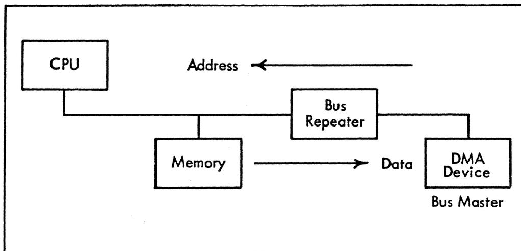
The Bus Repeater switches signal flow direction for various signals at precise phase times during cycles to ensure proper timing relationships between Q-bus signals. This is accomplished by an array of logic elements in the Repeater which monitors bus control signals and issues gating commands to several independent receiver and driver structures (see Figure 2).
