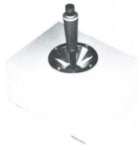
corresponding to the angular position of the joystick. The digital output controls the X and Y translation rates of the screen cursor.
