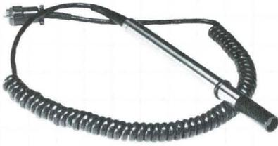
system for the selection of graphics elements. The pick module reads vector information off the Graphics Bus and provides data which relates displayed vectors to the actual display list. Picking may identify all or just parts of a graphic element. On stroke refresh displays a light pen or digital
