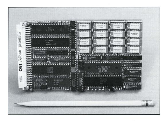
The Megatel Quark/150 is a low cost color graphics single 6 MHz board computer. The hardware features include 128K DRAM, Z80®, two serial ports, four parallel ports, floppy disk controller and of course the RGB color video output. All these features are packed into a tidy  $4" \times 6"$  Eurocard format.
