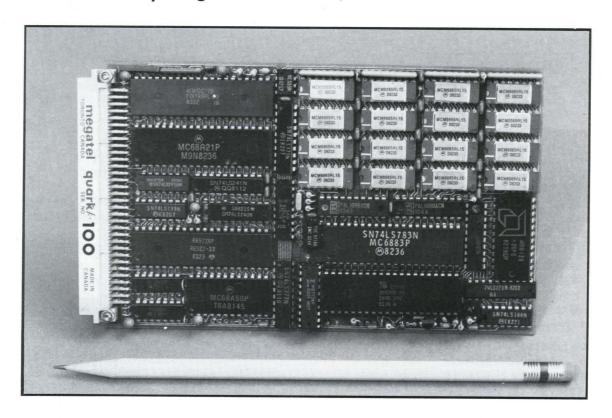
By utilizing PAL technology, Megatel's engineers have incorporated all of the most necessary elements for a CP/M® microcomputer on a small  $4'' \times 6''$  PCB — CPU, RAM, boot PROM, modem port, serial or parallel printer ports, parallel keyboard port, two general purpose parallel ports, floppy disk controller, and most importantly, the video display interface.
