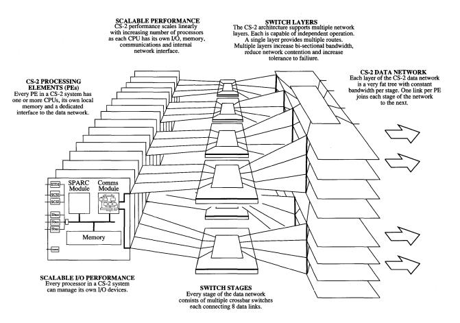
The distributed memory architecture guarantees a constant ratio of CPU performance, to memory and I/O bandwidth whatever the size of system giving scalable, balanced system performance.
