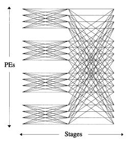
The CS-2 architecture supports up to 8 independent layers of this switching network, 1 layer being sufficient to achieve full connectivity with multiple routes. Current CS-2 systems use 2 of the 8 layers. They are engineered to expand to use all 8, giving a 256 element network a peak bi-sectional bandwidth of 102 GBytes/s.
