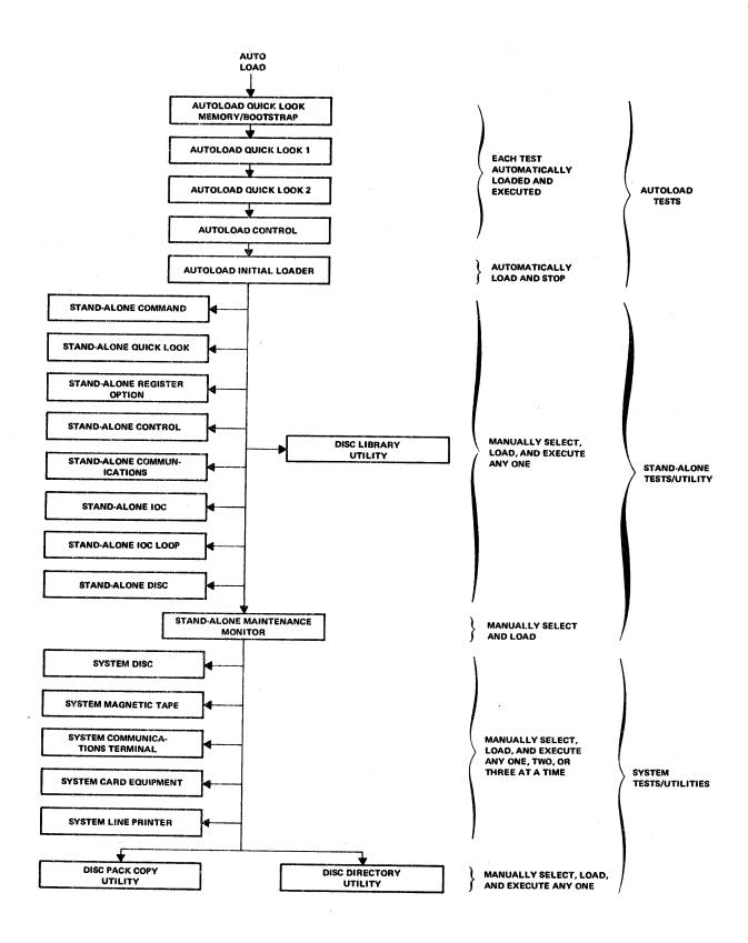
Figure 3-1. Machine Language Tests and Utilities on the DSD
