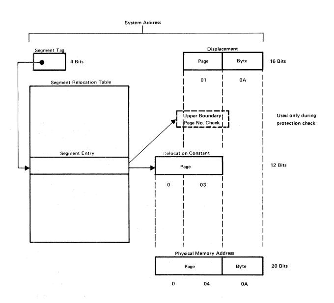
Figure 2-2. Generating Relocation Address
