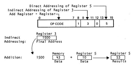
Indirect addressing applies to register numbers and memory addresses in the same way that direct addressing does. Bits 8 and 12 are associated with R1 and R2 for 2-byte instructions, with M1 and R2 for 4-byte instructions, and with M1 and M2 for 6-byte instructions. Indirect addressing is not allowed for 8-byte instructions. The following example of a 6-byte instruction shows how indirect addressing works in combination with indexing.
