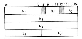
FUNCTION: The product of operand 1 (the multiplier) and operand 2 (the multiplicand) replaces operand 2. The multiplier size is limited to 253 digits and sign and also must be less than the multiplicand size. The length code,  $L_1$ , of the multiplier, if larger than 127, or greater than or equal to the length code,  $L_2$ , of the multiplicand is recognized as an overflow and no product is formed.
