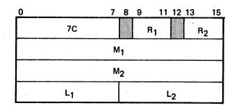
$\overline{\text{FUNCTION}}$ : Operand two, the dividend, is divided by operand one, the divisor, and replaced by the quotient and remainder.
