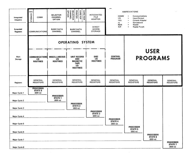
Figure 2-1. System Architecture
