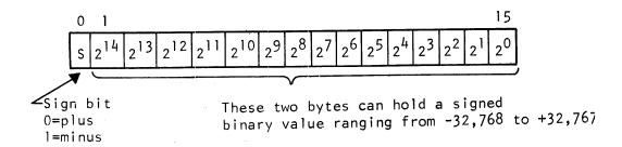
To determine the decimal value of a binary field, the decimal equivalents are added for each bit position that is on (1).
