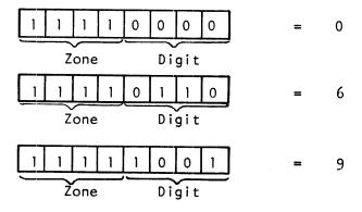
Since each digit requires a byte, a three-digit field requires three bytes, a seven-digit field requires seven bytes, and so forth. The number 10 would occupy two bytes.
