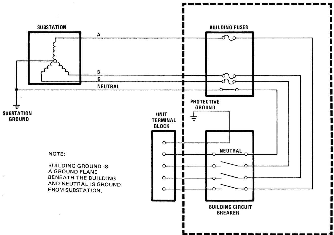
Figure 4-2. 50 Hz Power Schematic
