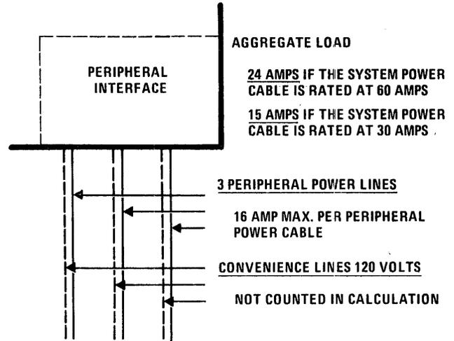
Figure 4-4. Power Distribution Facility Peripheral Interface
