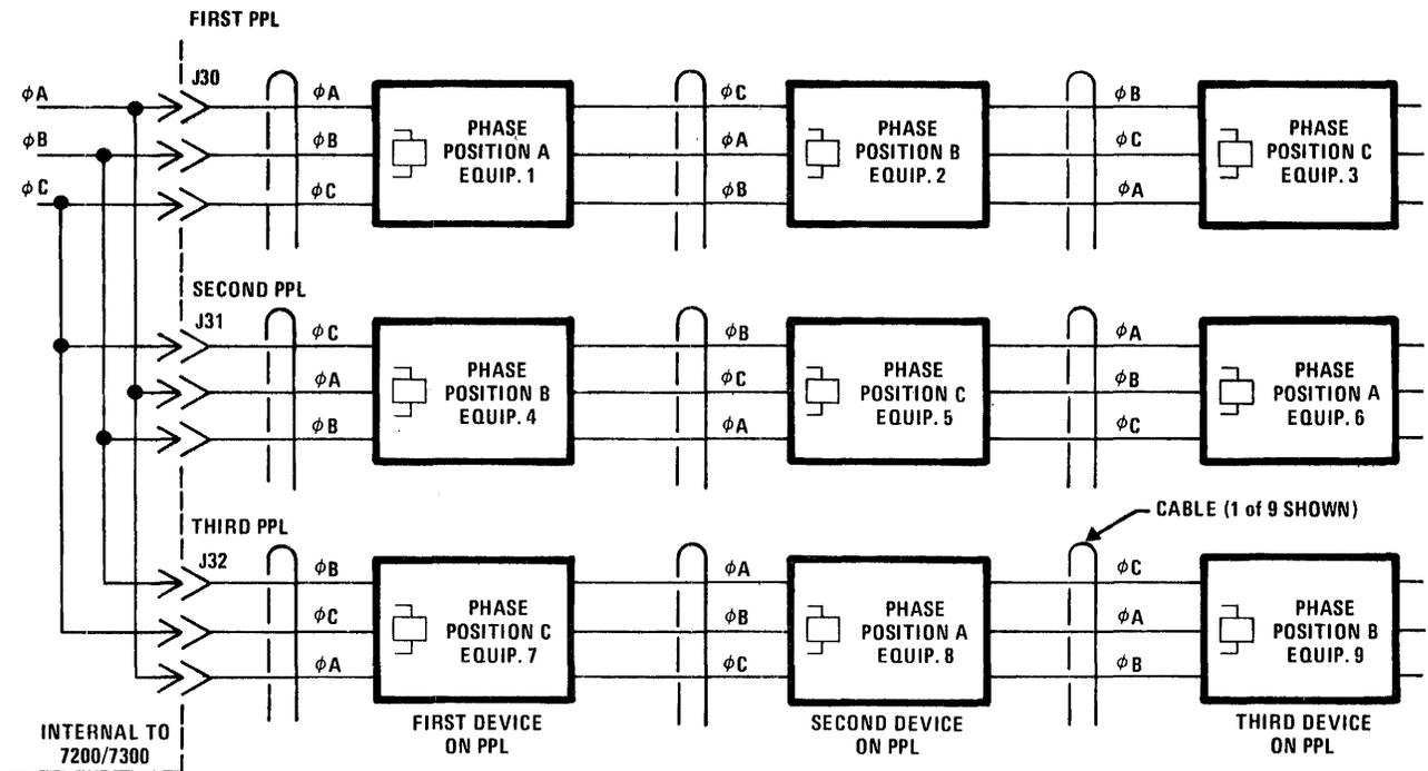
Figure 4-5. Power Phasing of Three PPLs
