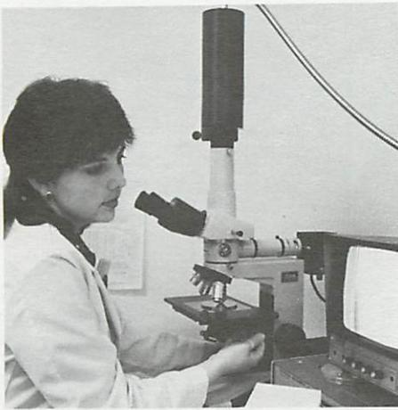
*This video measuring system is used to determine the thin-film head track width from pole to pole on each head contained on individual wafers.*
