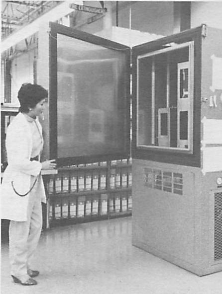
Individual integrated circuits and assembled printed circuit boards are "burned in" at high temperatures. This testing ensures that components will hold-up even under unusual stress situations.
