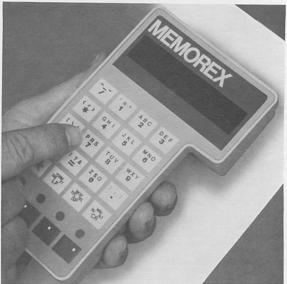
*One of the 3680's unique features is a hand-held portable maintenance terminal (PMT). This terminal is used to monitor performance and diagnose operational problems. "Previously, some units would have a diagnostic panel or interface the size of a suitcase," says Bill Brown, vice president for development engineers.*
