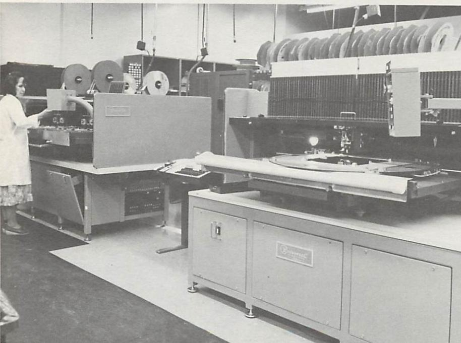
*(Top) Receiving many reels of standard PCB components, a single reel is produced by this computerized sequencer machine. The machine is programmed to arrange the components, in a specific logical order, for use on the automatic insertion equipment. (Bottom) These automatic insertion machines are programmed to place components on the blank PC boards.*
