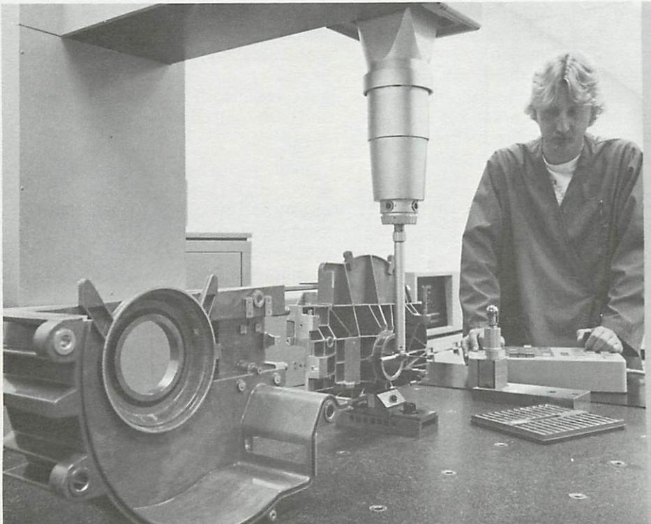
*The mechanical precision of every critical part of the 3680 HDA is checked. This state-of-the-art precision measurement system is accurate to as precise as 60 microns.*
