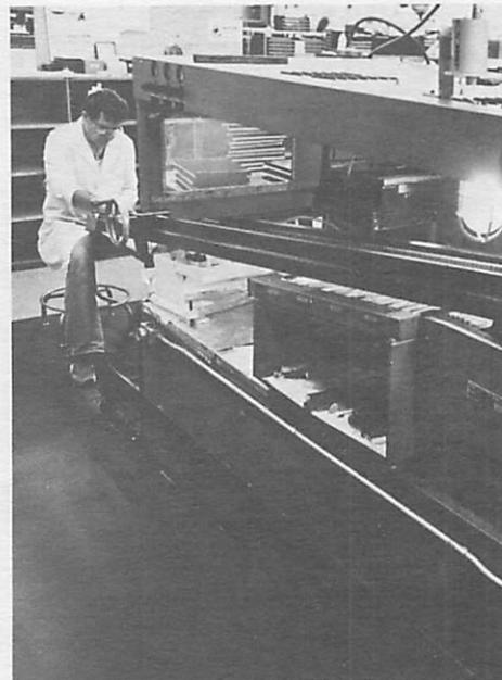
*As the PCB passes through the wave-solder system liquid solder connects the components to the board. Each board is visually inspected before it is sent through the cleaning and drying system.*
