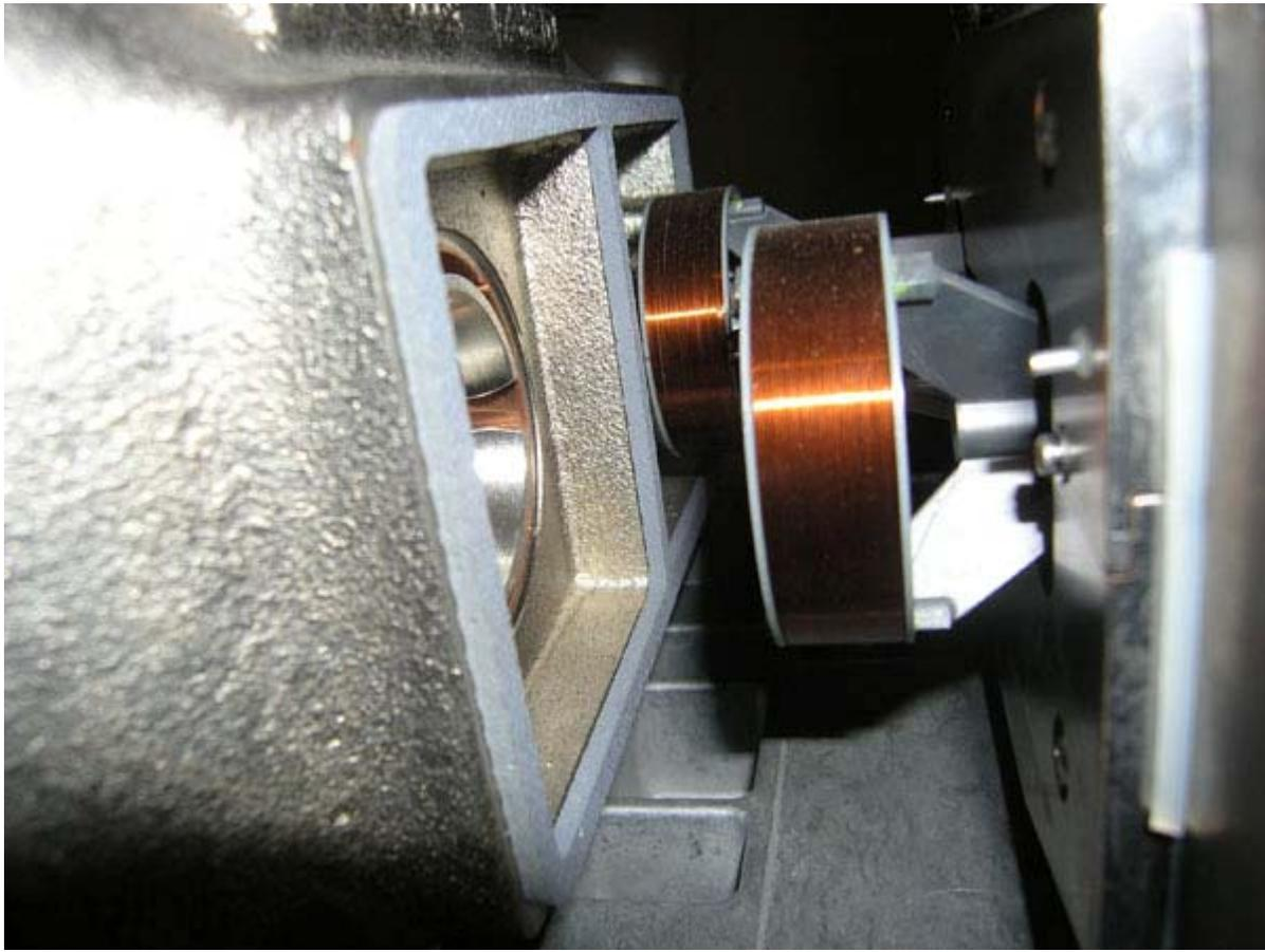
Here is the two head assembly voice coils. The two voice coils are out of their magnetic actuator motors (on the left) because the head disk assembly has been released to a position where it can be removed from the drive.
