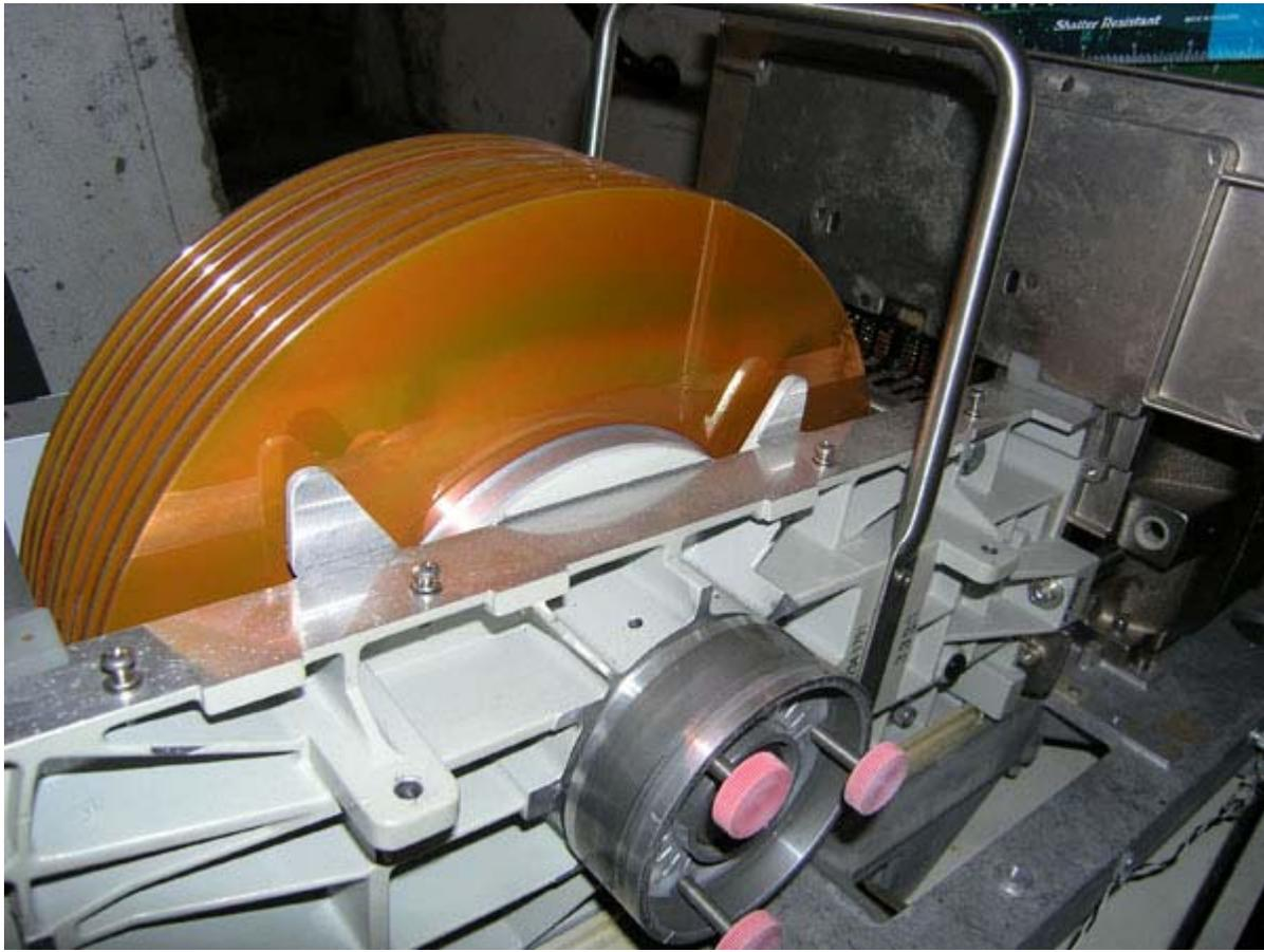
Here is a view of the 8 disk platters, giving 14 recording surfaces, plus two servo surfaces.
