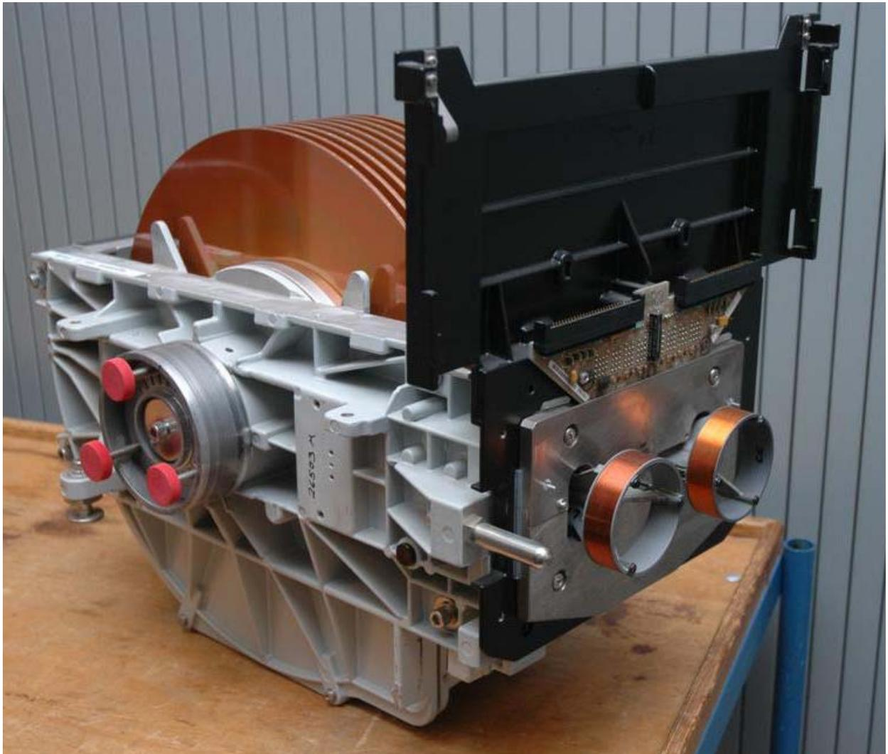
The Memorex 3680 Head Disk Assembly removed from the disk drive.
