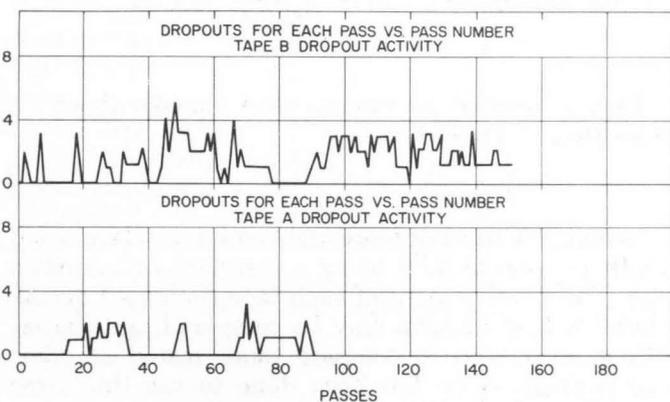
Figure 4. Drop-out activity plot — old method. Total wear length equivalent to 90 KHF.
