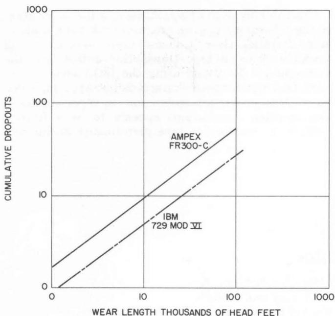
Figure 7. Drop-out Activity vs. wear length comparison using two tape transports with a single tape sample — data equally scaled for format and error differences.
