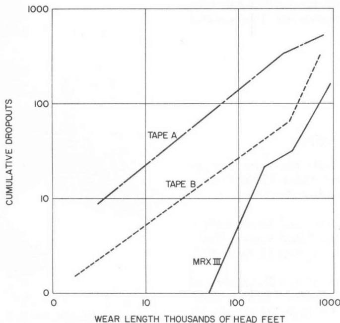
Figure 8. Drop-out Activity vs. wear length using full reel 2450 foot passes. Each curve represents a type of precision computer tape.
