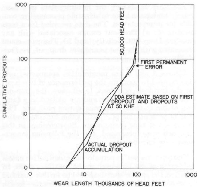
Figure 5. Drop-out accumulation vs. wear length. Durability, Drop-out Activity three point estimation vs. point by point plot.
