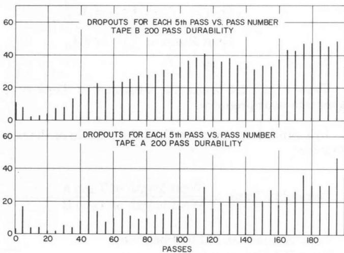
Figure 3. Full reel pass durability plot — old method. Total wear length equivalent to 500 KHF.
