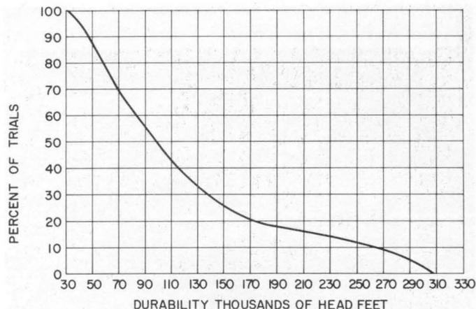
Figure 2. Durability variation as a function of trials. Control tape durability measured on the same transport during a 3 months interval.
