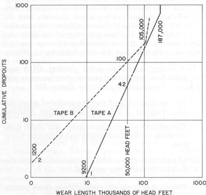
Figure 6. Cumulative drop-outs vs. wear length. Comparison presentation of two computer tapes for Durability, Drop-out Activity analysis.
