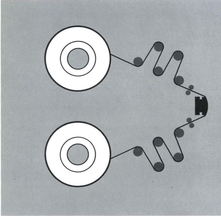
Mechanical Buffering-Tension (Compliance) Arm
