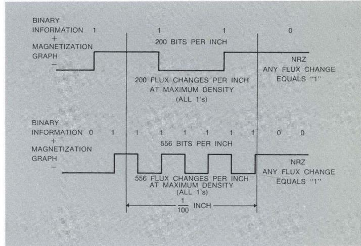
DIGITAL INFORMATION IS RECORDED ON MAGNETIC TAPE BY MAGNETICALLY SATURATING THE TAPE IN ONE DIRECTION OR THE OTHER
