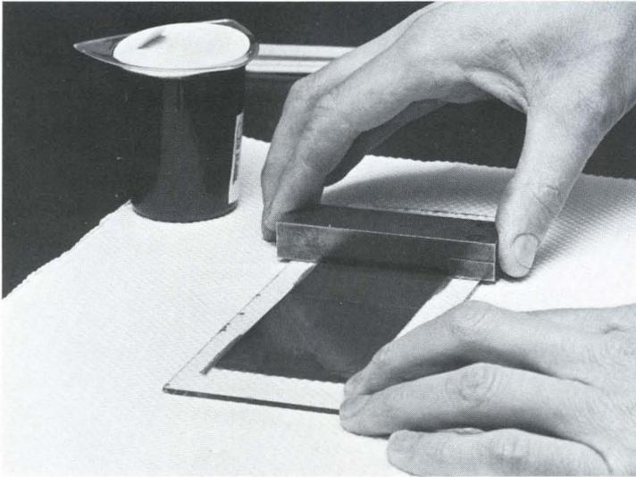
Dispersing Factors. Draw down test is used to maintain continuous quality control during the dispersion operation.
