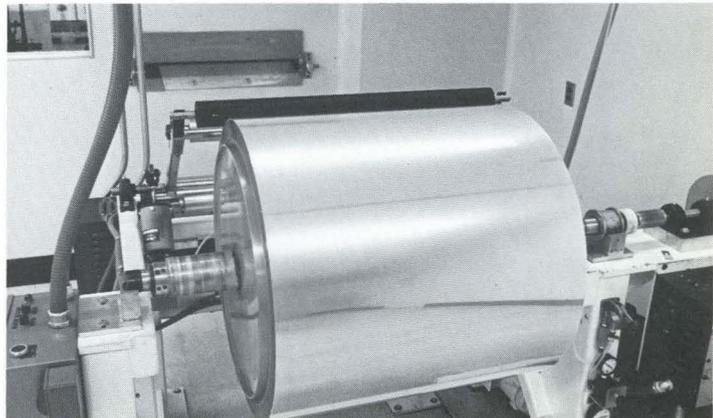
Polyester jumbo rolls are ultrasonically cleaned and transferred into clean room.
