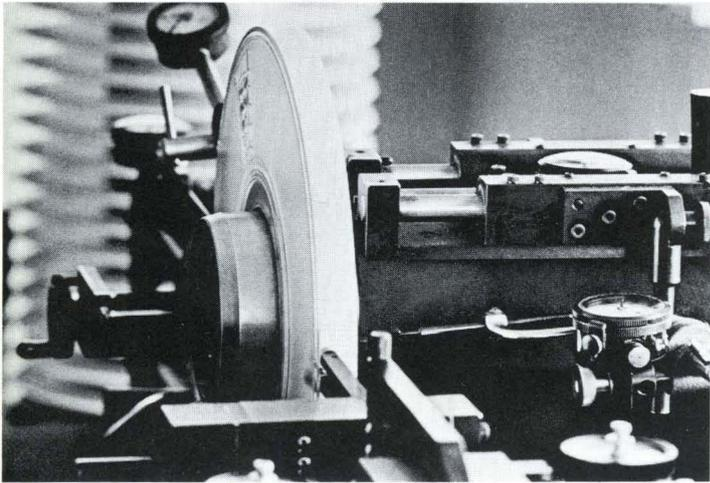
Four critical flange measurements are checked.
