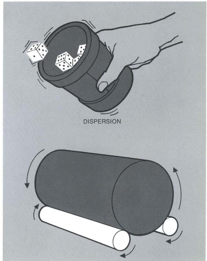
The Dispersing Techniques. The violent shaking and interaction of dice in a dice cup is a good illustration of the concept of mechanical dispersion. Very high shear forces are developed using solid dispersing media.
