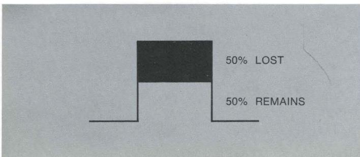
Dropout profile when the computer clips at 50%.
