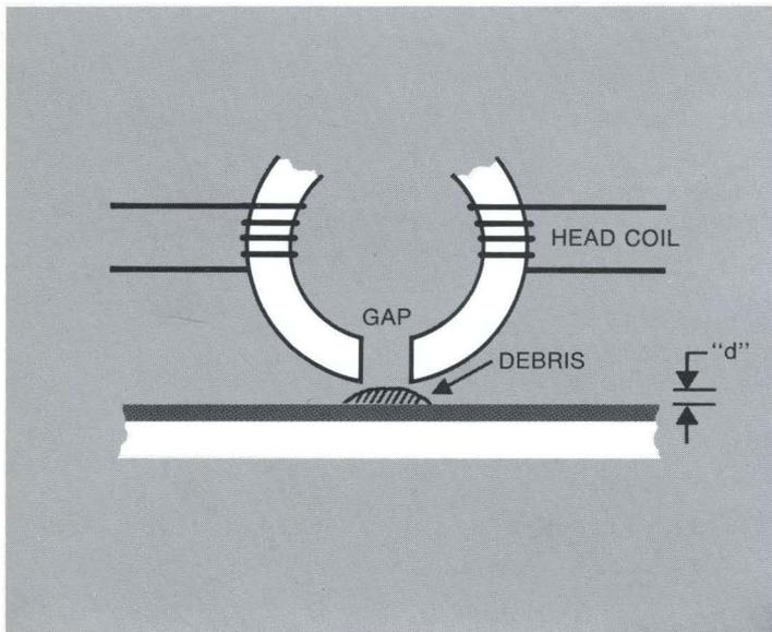
Debris causes head to tape separation.
