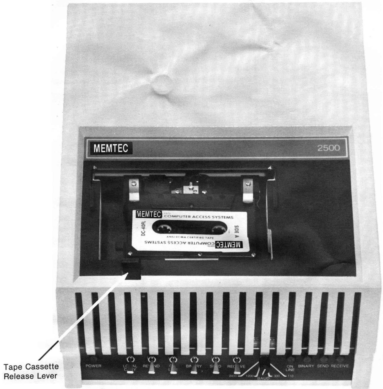
Figure 3-5: Tape Cassette Release Lever
