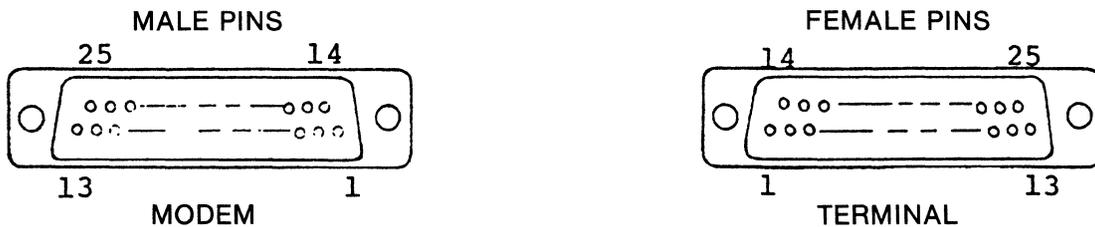
Figure 2-6: I/O Connector Mechanical Layout
