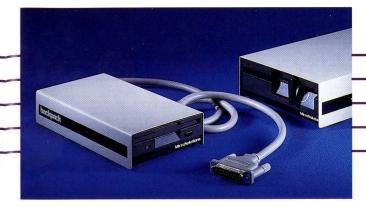
Adding a disk drive has never been this easy. The **backpack** external floppy drive plugs into your parallel printer port. There are no interface cards to install, so you don't have to open the cabinet of your computer.
