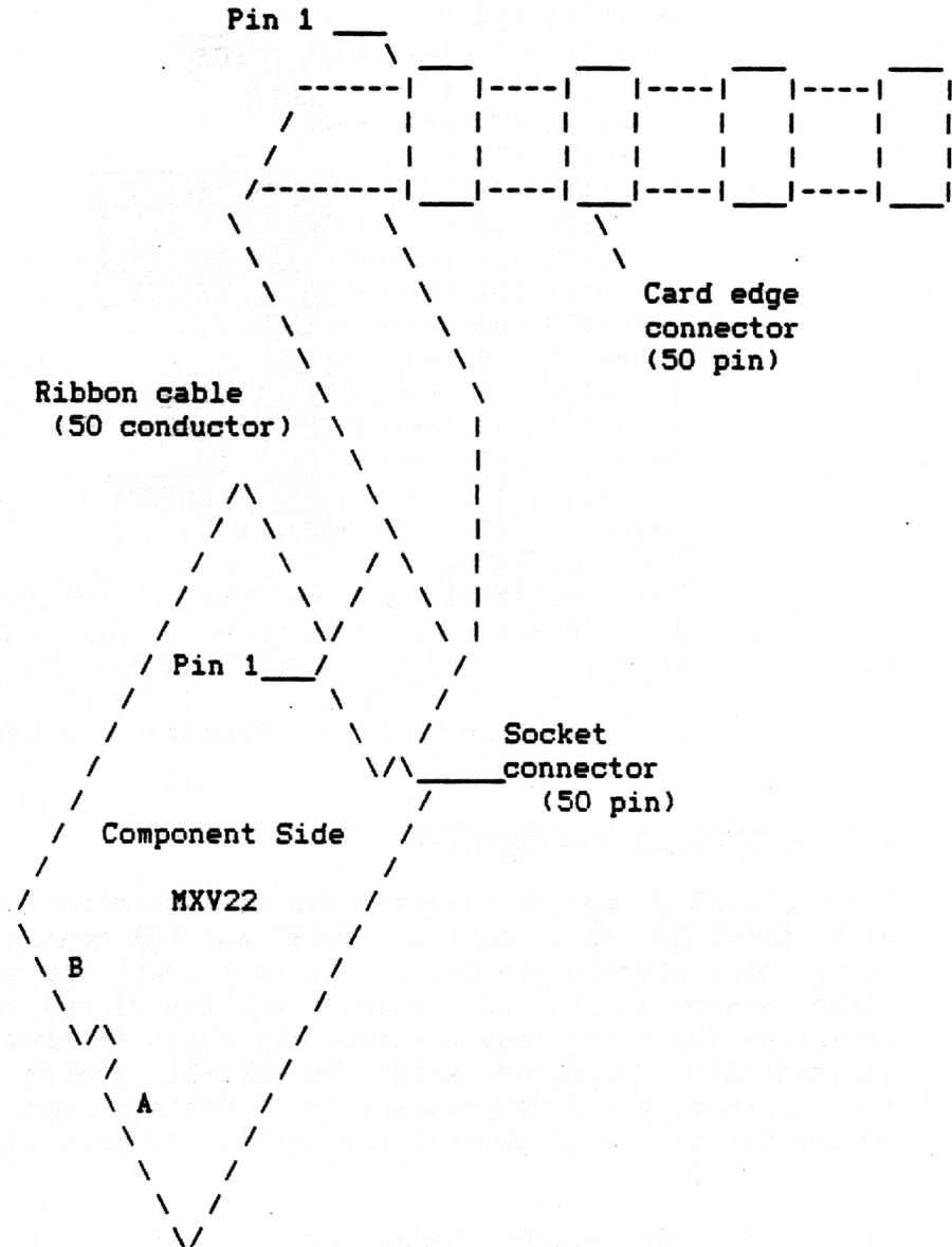
Figure 2-2: Drive/Controller Cabling
