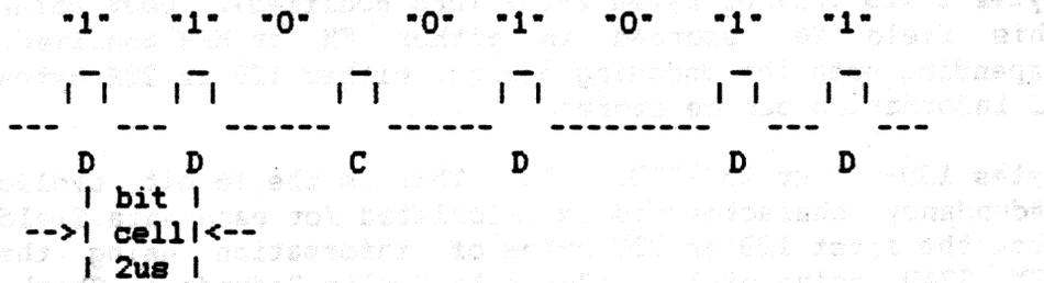
**Figure 1-3: MFM Recording Characteristics**
