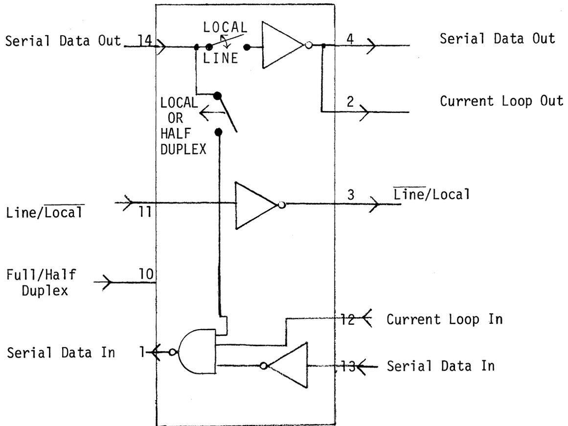
Figure 4.1: CR2 Functional Diagram
