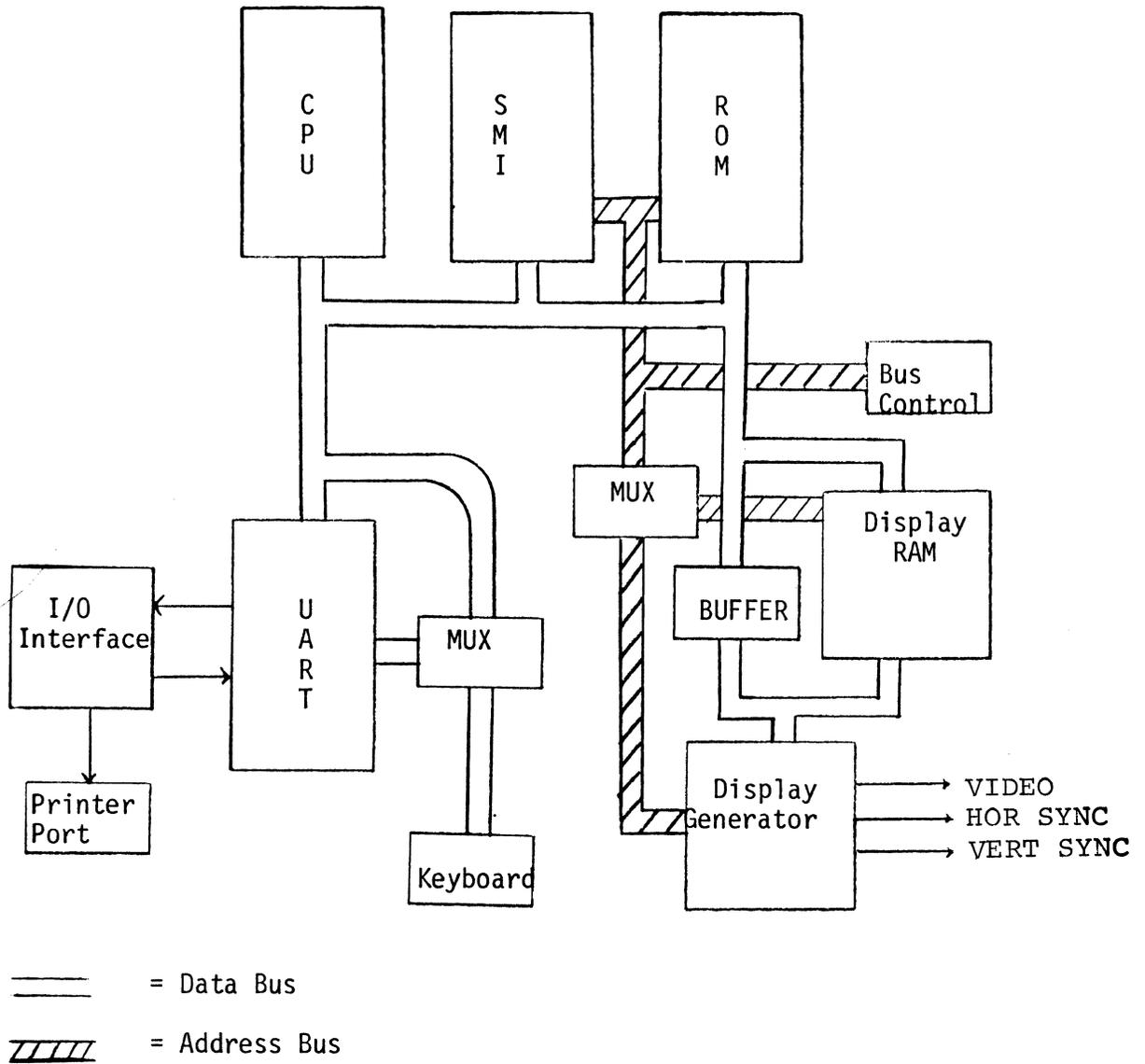
Figure 1.1: MIME-I Block Diagram
