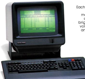
Each ERGO terminal features a detached, low profile keyboard with integrated palm rest, hidden tilt mechanism which allows the user a full 25 degree change in viewing angle. P31 green display with brightness control from the keyboard, screen saver, volume control for bell and keyclick loudness, and an on/off switch up front—where you can reach it.
