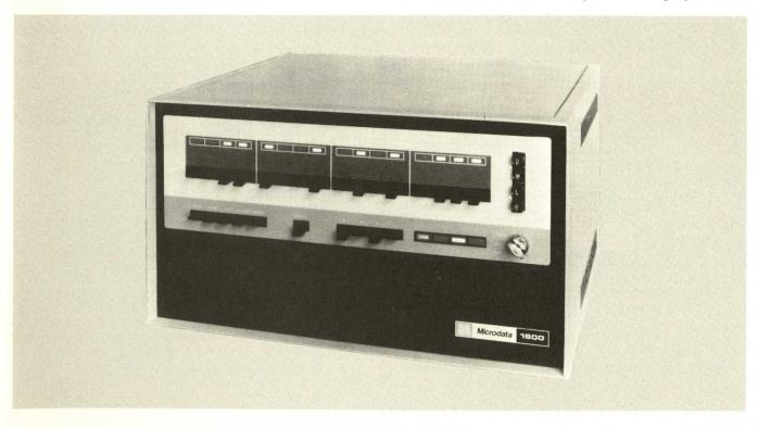
BASIC, COBOL, FORTRAN, SNOBOL, ATLAS or equivalent. Utilization of large arrays of high-speed read-only memory for language implementation eliminates intermediate compile operations and results in an interpretive processor with compile-and-go capability in the machine at all times.
