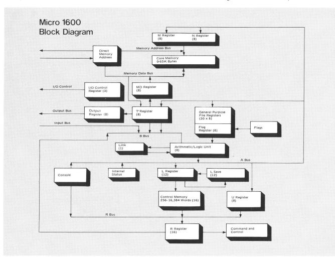
program: the MD register buffers T during memory write cycles; the output register buffers T during I/O data output operations.
