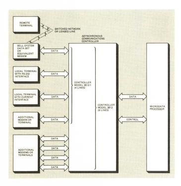
The flexibility of the Asynchronous Communications Controller provides the Microdata processor with many local and remote data communications options.
