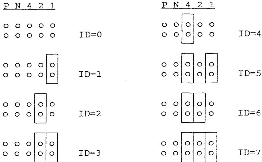
A jumper is installed on "P" to enable parity. Parity is never used with an SB180/SB180FX. "N" has no connection.
