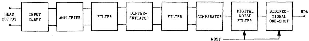
Figure 3-16. Read Channel Block Diagram
