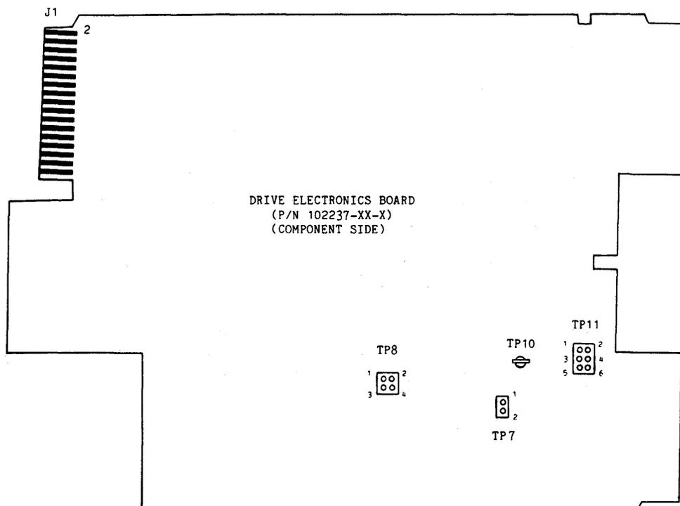
Figure 4-1. PCBA-Mounted Components
