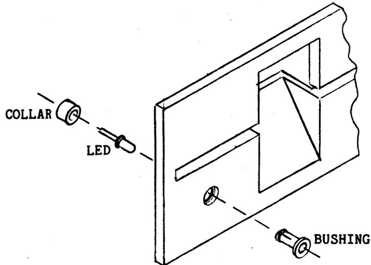
Figure 6-22. In-Use LED Assembly
