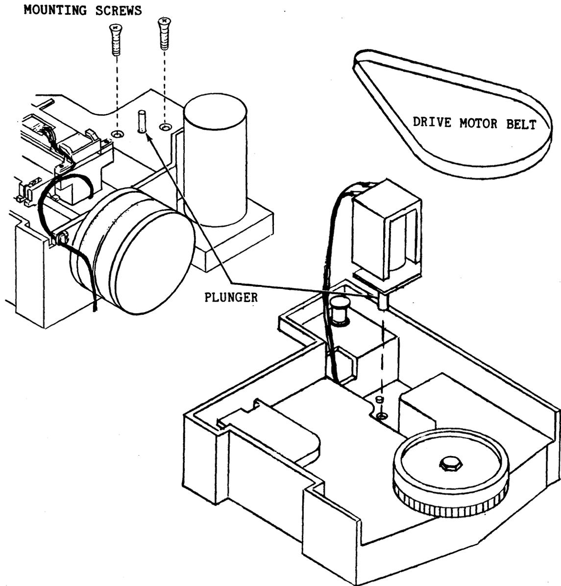
Figure 6-11. Head Load Solenoid
