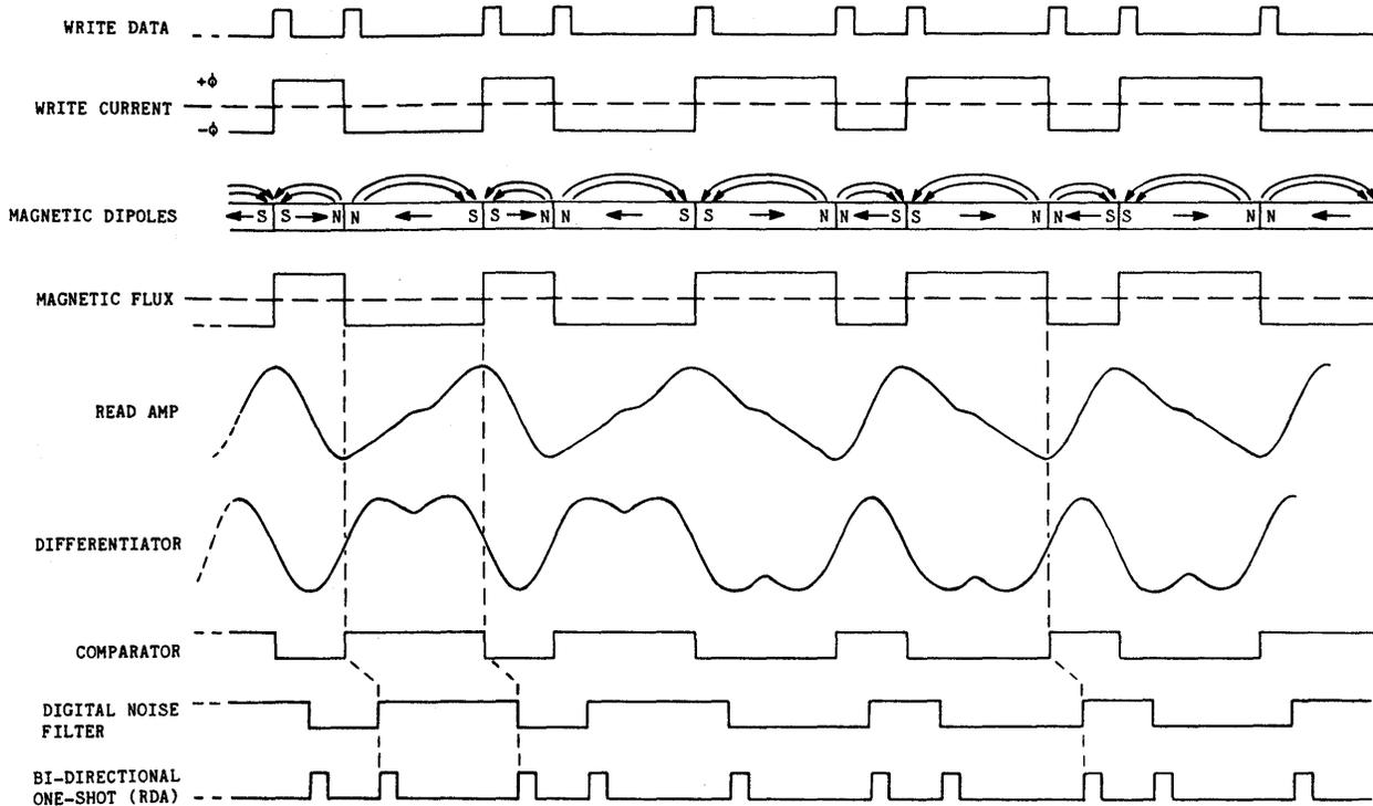
Figure 3-14. Recording Process - Detailed
