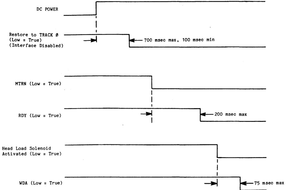
Drive functions are unavailable to the user until the initialization is complete; i.e., TRK0/ is true.
