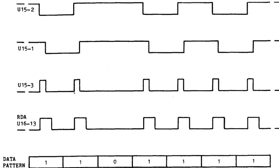
Figure 3-18. Bidirectional One-Shot Timing Diagram
