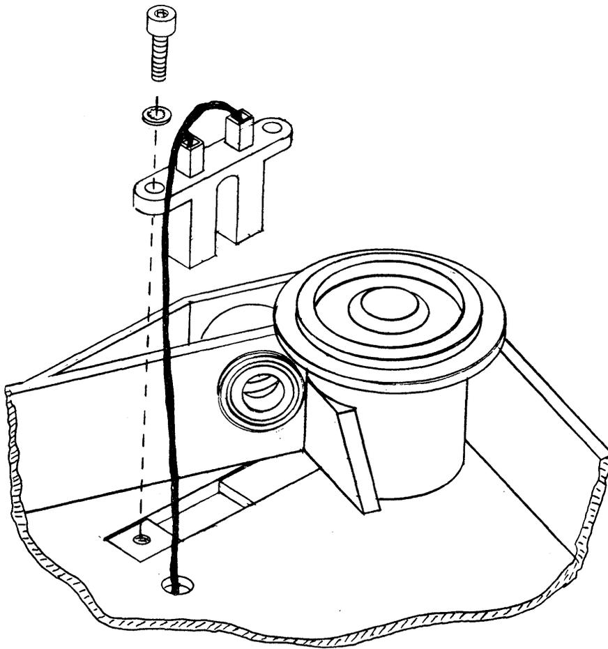
Figure 6-14. Tach Sensor Placement
