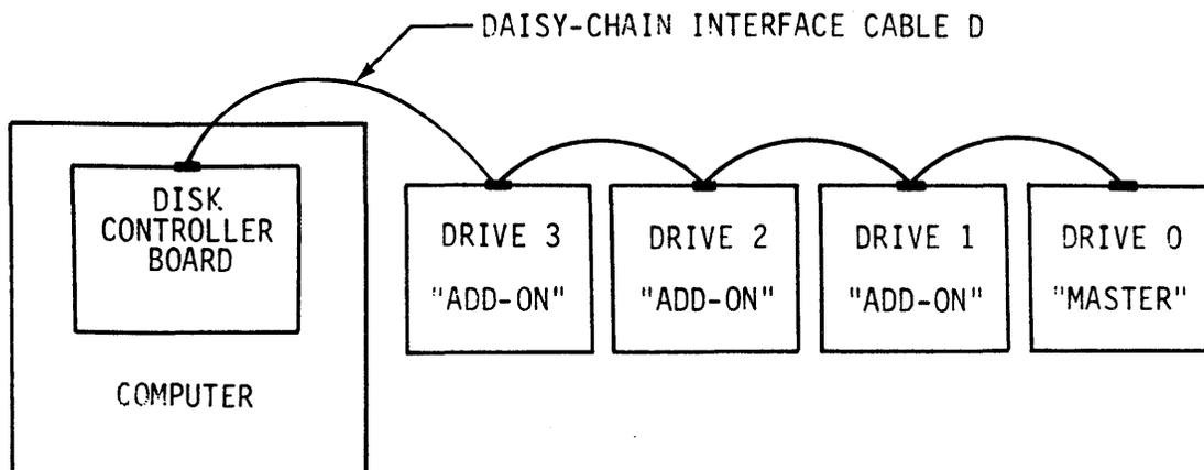
Figure 2-2. Typical Multiple Drive System
