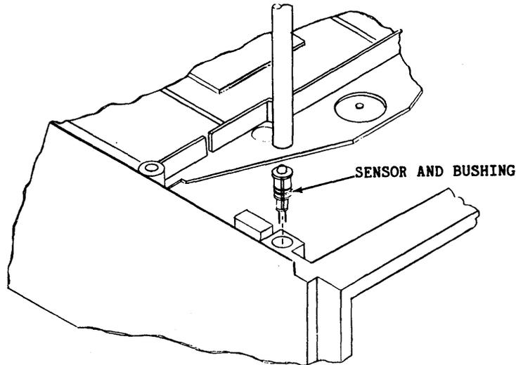
Figure 6-21. Write Protect Sensor Assembly
