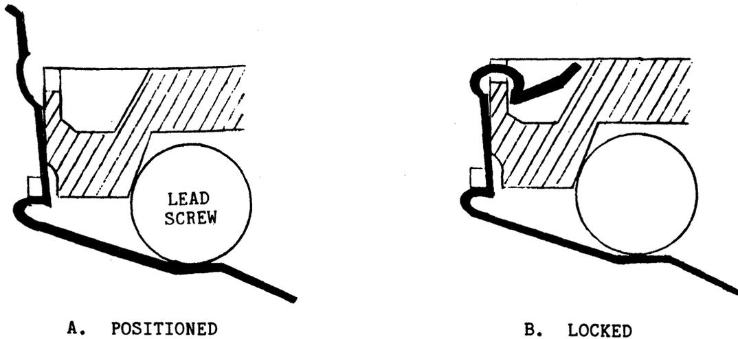
Figure 6-9. Carriage Spring Placement
