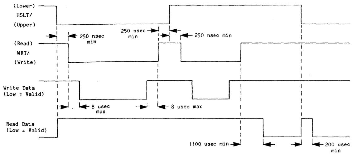
Figure 3-10. Head Select and Read/Write Control Timing
