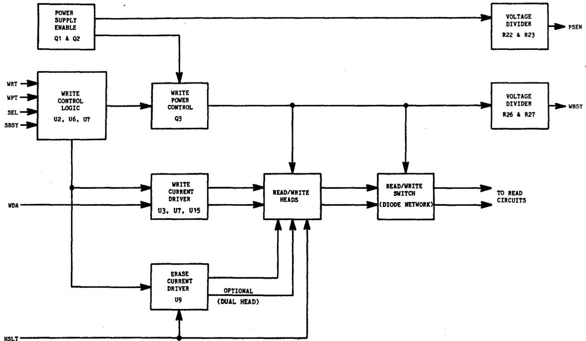
Figure 3-15. Write Channel Block Diagram
