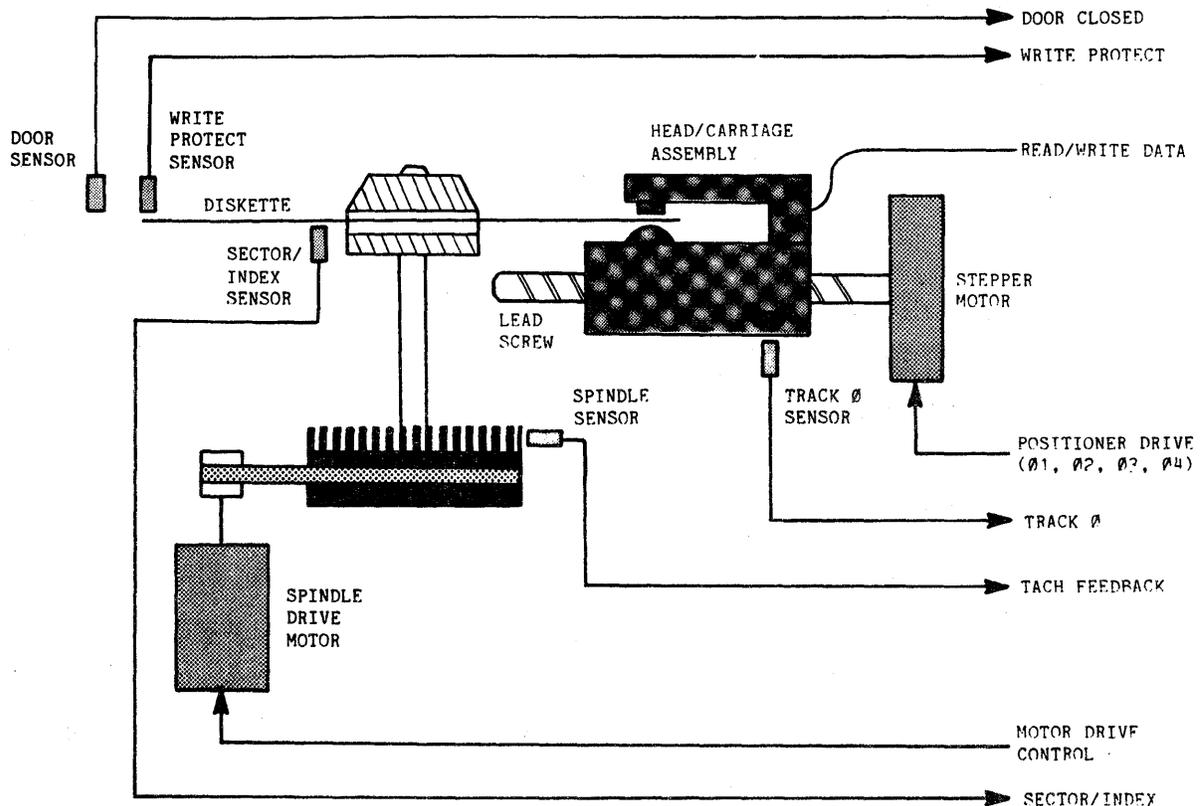
Figure 3-2. Drive Mechanical Elements
