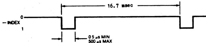
Figure 2-11. Index Pulse Timing
