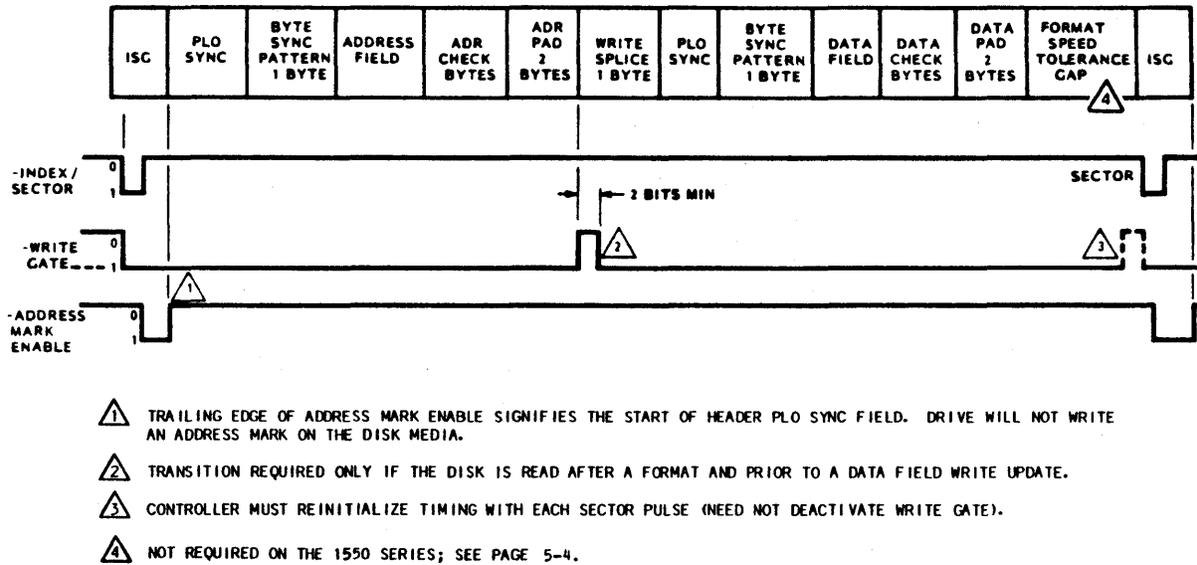
Figure 5-2. Fixed Sector Address Mark, Write Gate, and PLO Sync Format Timing
