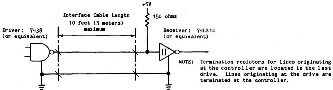
Figure 2-1. Control Signal Driver/Receiver Combination
