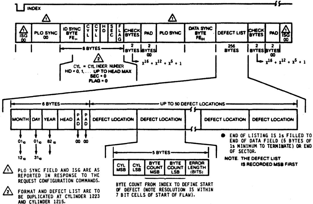
Figure 5-6. Defect List Format
