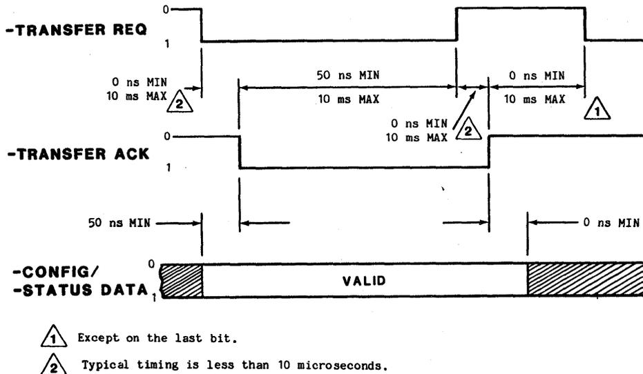
Figure 2-5. One Bit Transfer Timing - From Drive
