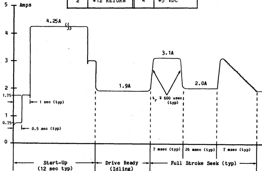
Figure 4-1. 12V Peak Current Profile (typical, 1558-15)
