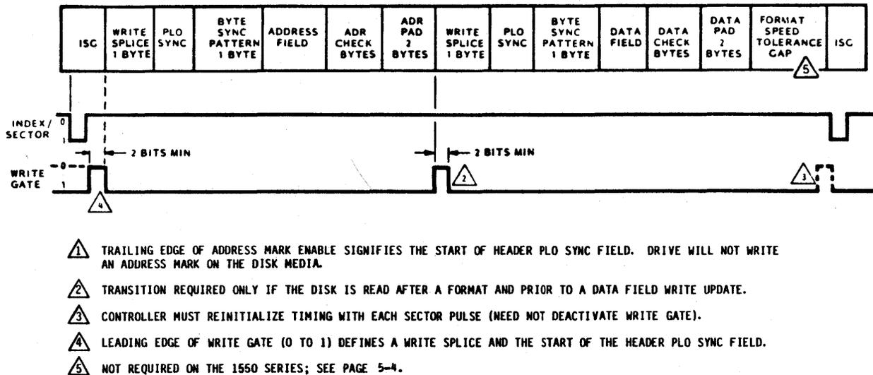
Figure 5-3. Fixed Sector Address Mark, Write Gate, and PLO Sync Format Timing (alternative method)
