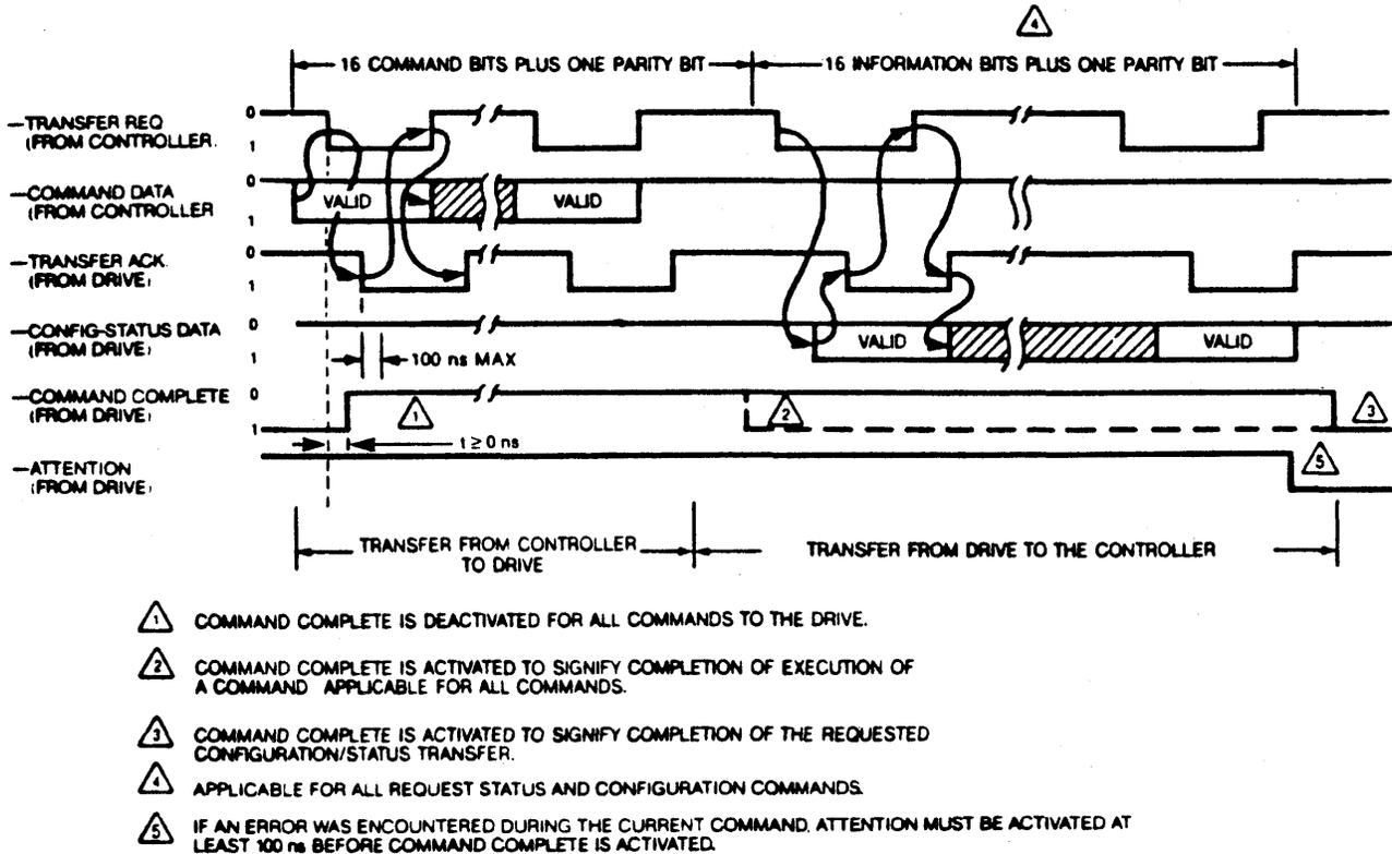
Figure 2-10. Typical Serial Operation(s)
