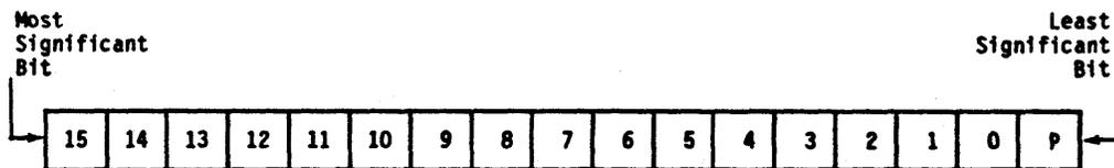
Figure 2-9. Configuration/Status Data Word Structure
