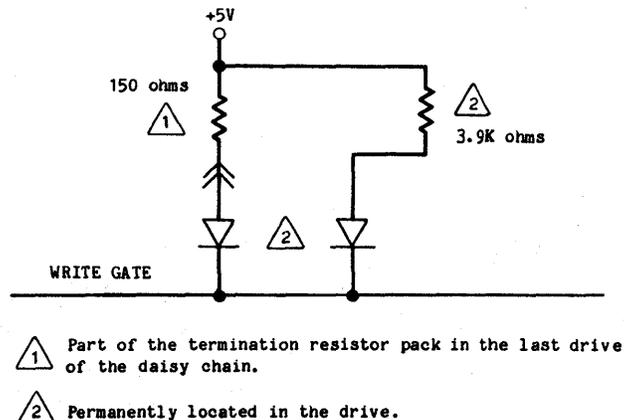
Figure 2-4. Write Gate Termination
