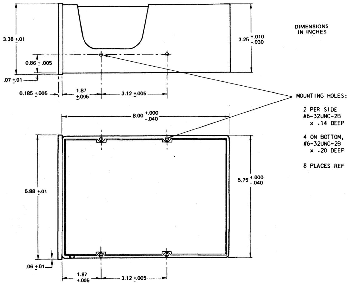
Figure 3-4. Dimensions and Mounting
