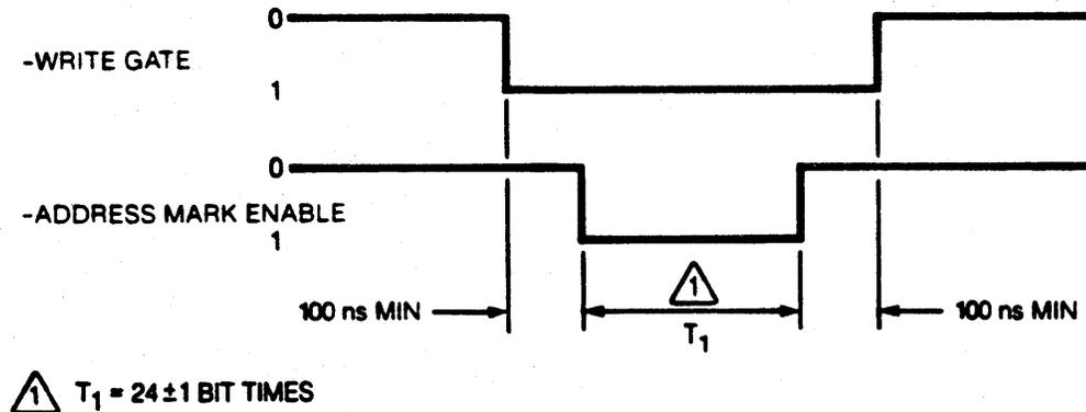
Figure 2-7. Write Address Mark Timing
