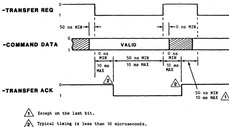
Figure 2-6. One Bit Transfer Timing - To Drive
