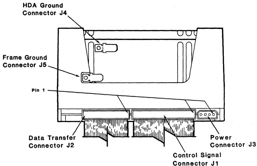
Figure 3-1. Power and Interface Connections
