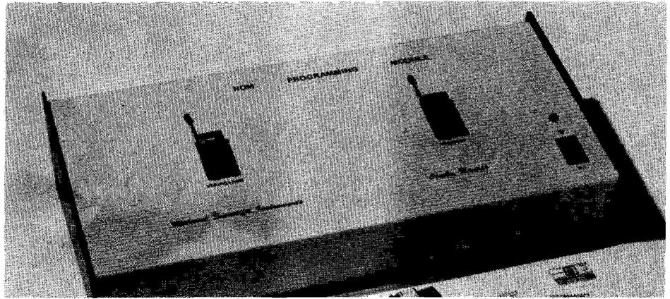
tion, the software reads the PROM back into memory and compares each step with the memory location from which it was programmed for the purpose of verification. Any discrepancies are listed on the terminal with an error message. If the PROM verification is correct, then a checksum
