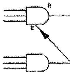
6.5 MULTIPLE FLIP-FLOP INPUTS. Multiple inputs physically integral with flip-flop functions are drawn as shown in Example 1, and so "tagged." Multiple inputs physically separated from the flip-flop functions are drawn as shown in Example 2, and separately tagged. See also Appendix A, figure 12.
