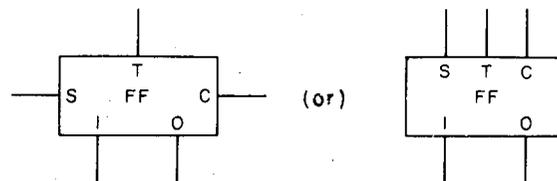
"S" input shall be in proximity to the "1" output. "C" input shall be in proximity to the "0" output. The aspect ratio of the symbol shall be 1.75 to 1. (See application examples in Appendix A.)
