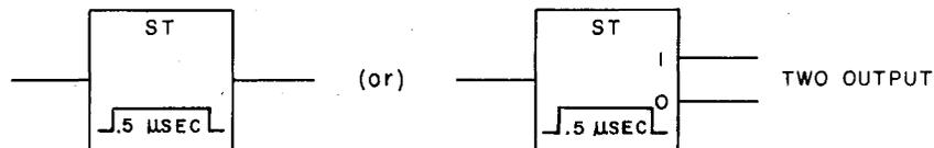
5.13 GENERAL LOGIC SYMBOL. Symbol for functions not elsewhere specified. The symbol shall be adequately labeled to identify the function performed. It is not intended that this symbol be used for functions which can be logically expressed by a single symbol established in this standard. Aspect ratio shall be 2:1 or greater.
