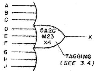
6.2 Multiple inputs to physically separated functions with common outputs.
