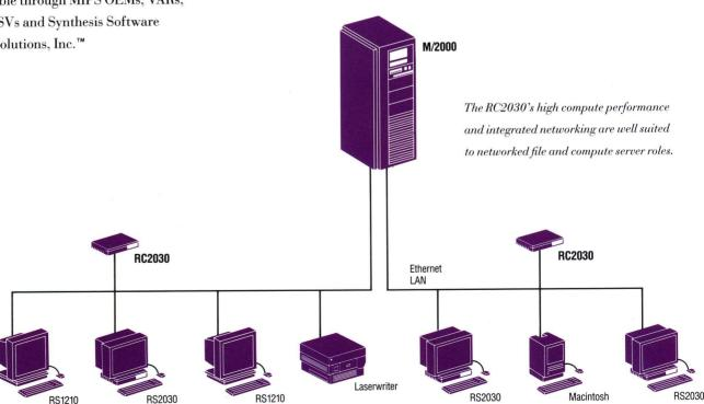
Optimized for price/performance and office operation, the RC2030 is a single-board computer housed in a compact desktop unit. The base unit has a small footprint, can accommodate two 3.5-inch half-height peripherals, and uses standard AC wall power. Optional desktop and deskside expansion units are available for additional media and disk capacity.
