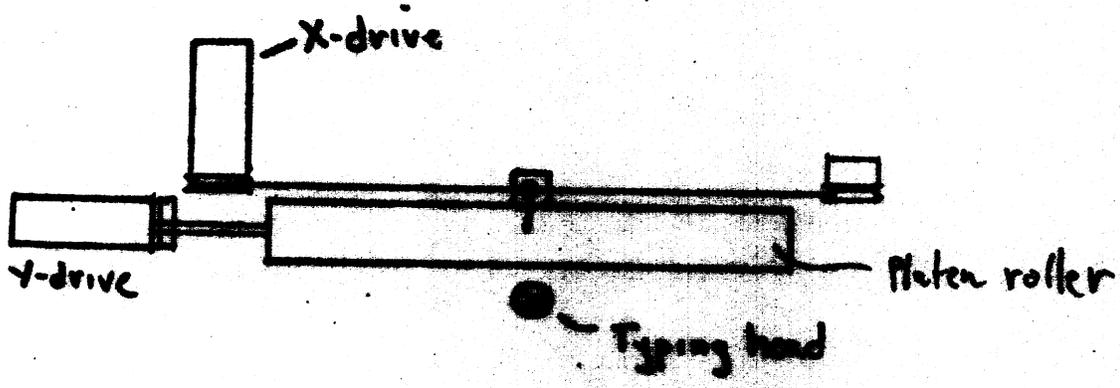
There will be some mechanical problems in making the reversible paper-feed reliable; the pen must write very close to the platen pinch-roller if a paper-tension system is to be avoided.
