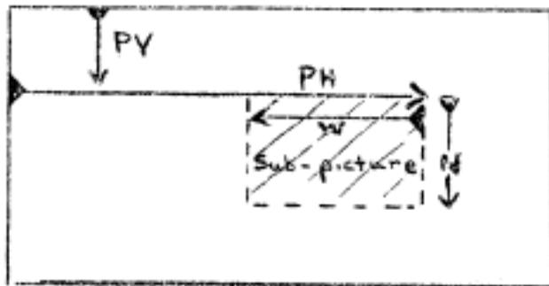
All pictures are composed of 36-bit groups of single-level digitized video. The basic function of the device is to read-in to the computer the contents of a 36-bit shift register that is loaded at a certain (programmable) rate from the video signal for each horizontal line.
