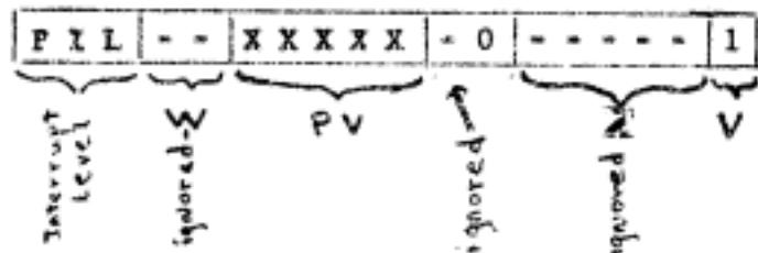
This will cause an interrupt on channel PIL when vertical position PV is reached. The parameters W, PH, and bit 10 have no effect. Bit 11 becomes set at interrupt time. Bit 17 determines whether the device is in vertical or horizontal select mode.
