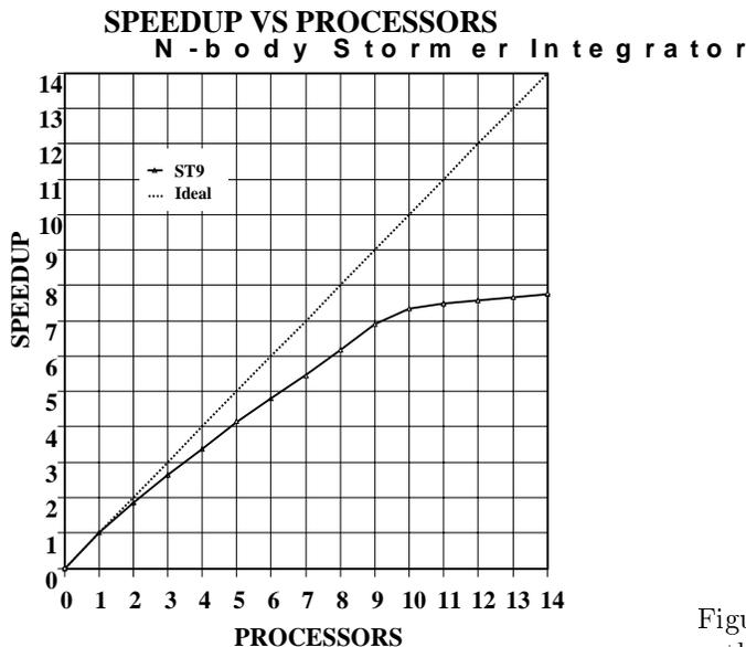
Figure 5: Speedup graph of Stormer integrations. Ample speedups are available to keep the 8-processor *Supercomputer Toolkit* busy. However, the incremental improvement of using more than 10 processors is relatively small.
