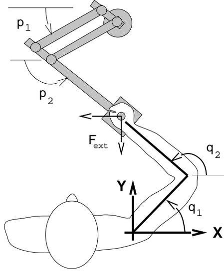
**Figure 1:** Sketch of the manipulandum and the experimental setup. Planar arm movements were made by the subject while grasping the handle of the manipulandum. A monitor, placed directly in front of the subject and above the manipulandum (not shown), displayed the location of the handle as well as targets of reaching movements. The manipulandum had two torque motors at its base which allowed for production of a desired force field.
