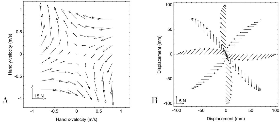
**Figure 3:** An environment as described by the force field in Eq. (1). **A:** The force field. **B:** Forces acting on the hand during simulated center-out reaching movements. Movements are simulated as being minimum-jerk with a period of 0.5 sec and amplitude of 10 cm.
