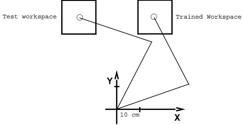
**Figure 2:** Configurations of a model two joint arm, representing typical kinematics of the human arm, at two workspace locations where reaching movements were performed. Typical shoulder and elbow angles at these two workspaces were 15 and 100 degrees at right and 60 and 145 degrees at left, using coordinates defined in Fig. 1.
