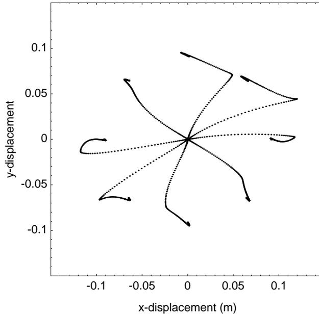
**Figure 12:** Simulated after-effect trajectories: Hand trajectories for the skeletal dynamics of Eq. (11) in a null force field with the controller of Eq. (12), assuming that the controller had formed an internal model of the force field shown in Fig. 3.
