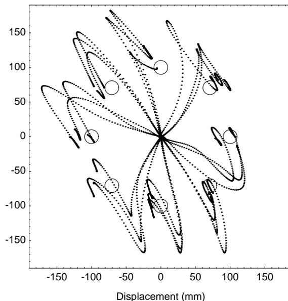
**Figure 7:** Performance during initial exposure to a force field: Shown are hand trajectories to targets at the right workspace while moving in the force field shown in Fig. 3. Movements originate at the center. All trajectories shown are under no-visual feedback condition. Dots are 10 msec apart.
