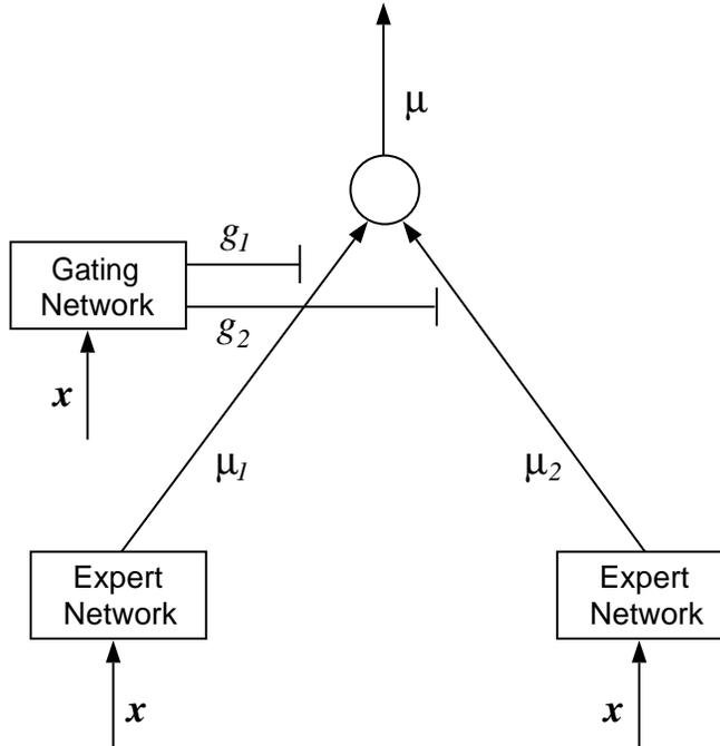
Figure 1: The mixture of experts architecture. The total output  $\mu$  is the weighted sum of the expert network outputs:  $\mu = g_1\mu_1 + g_2\mu_2$ , where the weights are the gating network outputs  $g_1$  and  $g_2$ .
